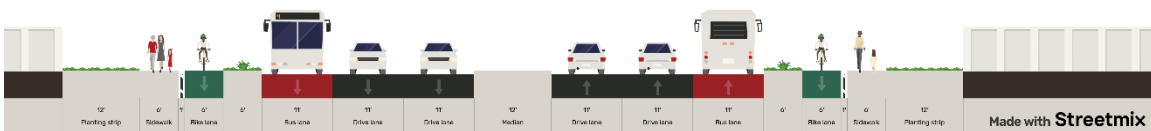
Figure 15: SR 99/SR 525 Interchange Proposed Typical Cross-section with Concept 2: Separated Bike Facilities – 130 foot ROW
