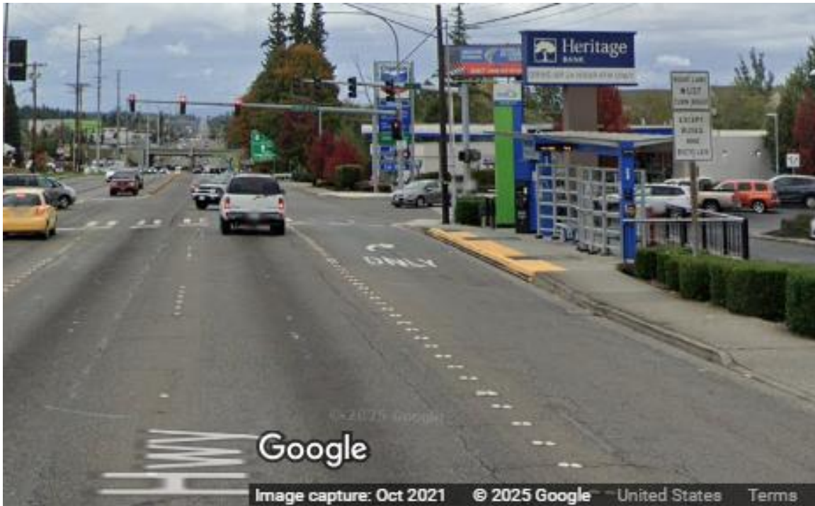
Figure 14: Current implementation of “right-turn only except for transit” on SR 99 northbound at 148th Street Southwest. Google Maps Street View
