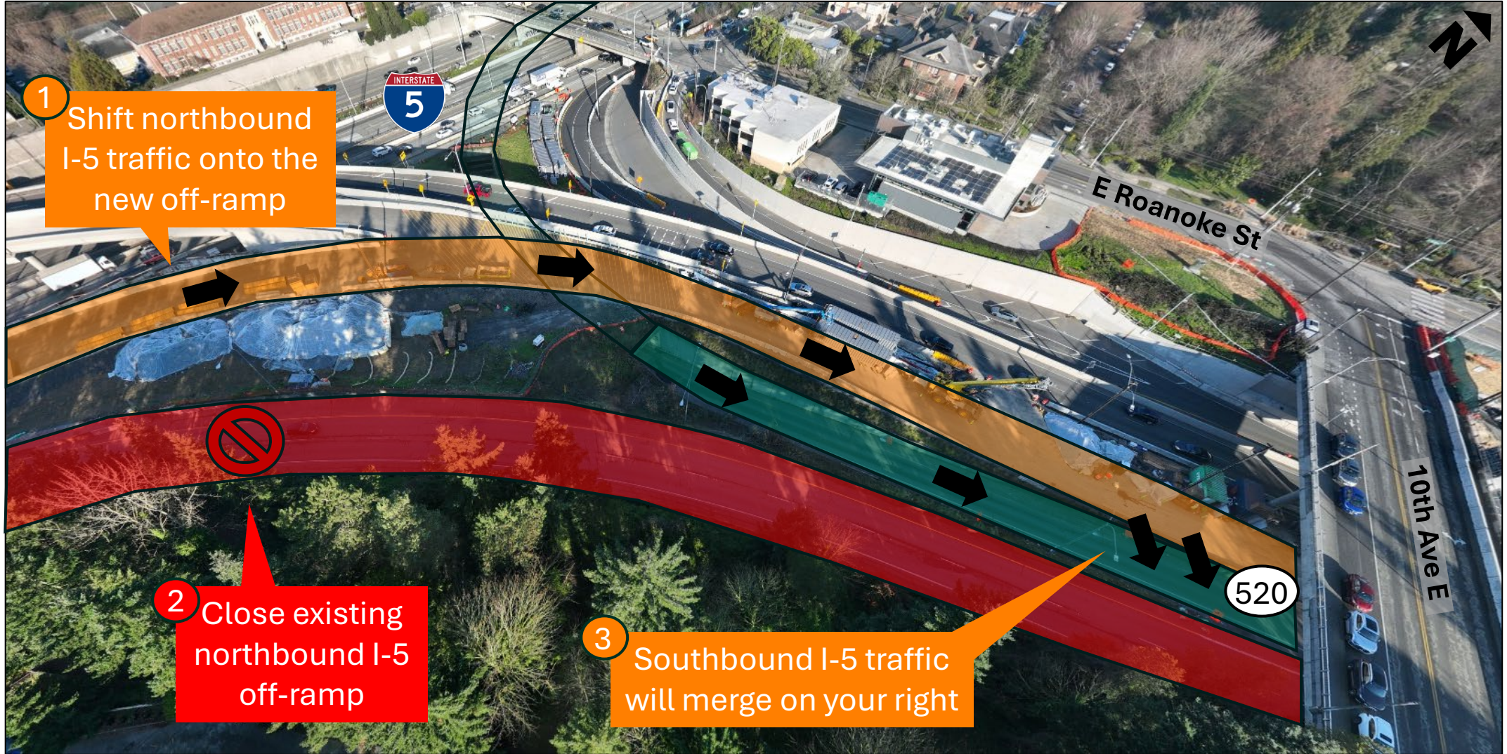
Map showing the upcoming changes to the northbound I-5 off-ramp to SR 520.
