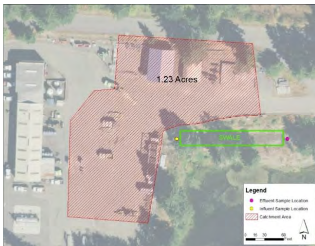
Figure 2. Mottman CABS monitoring site and associated drainage
