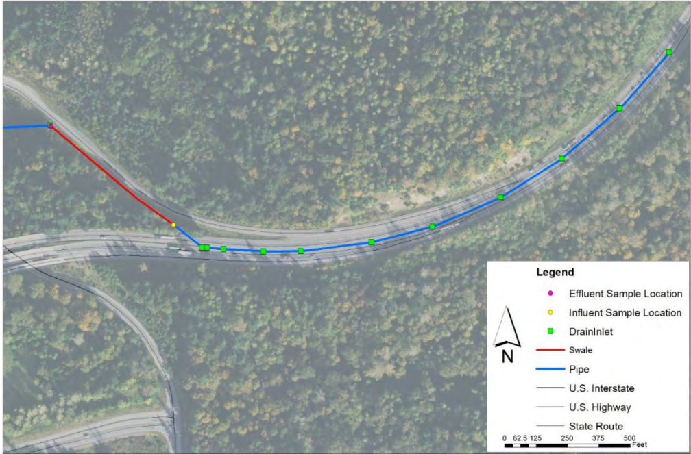
Figure 5 Mirrormont biofiltration swale monitoring site and associated drainage features
