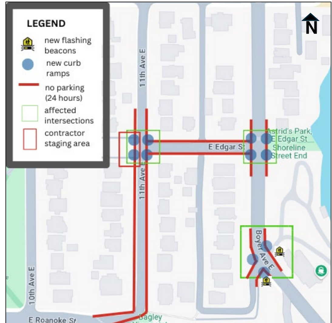
Map of the curb ramp upgrades (Photo/SDOT).
