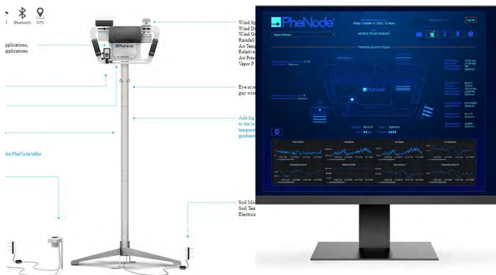
Figure 13-14: The PheNode system enables monitoring of soil moisture, soil temperature, and electrical connectivity; data collection of wind speed/direction, gusts, rainfall, air temperature, relative humidity, air pressure, and vapor pressure; and takes photos.
