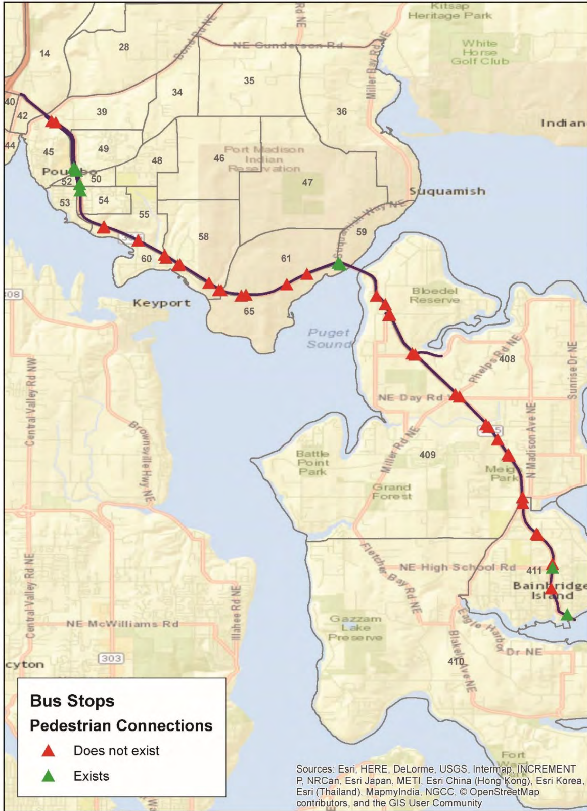
Figure 11. Existing Pedestrian Connections to Transit Stops on SR 305
