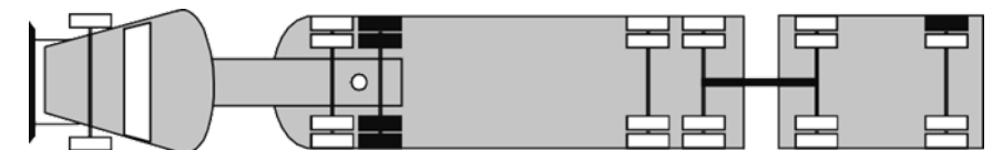
All tires on one drive axle and one tire on either side of the last axle of the last trailer.
