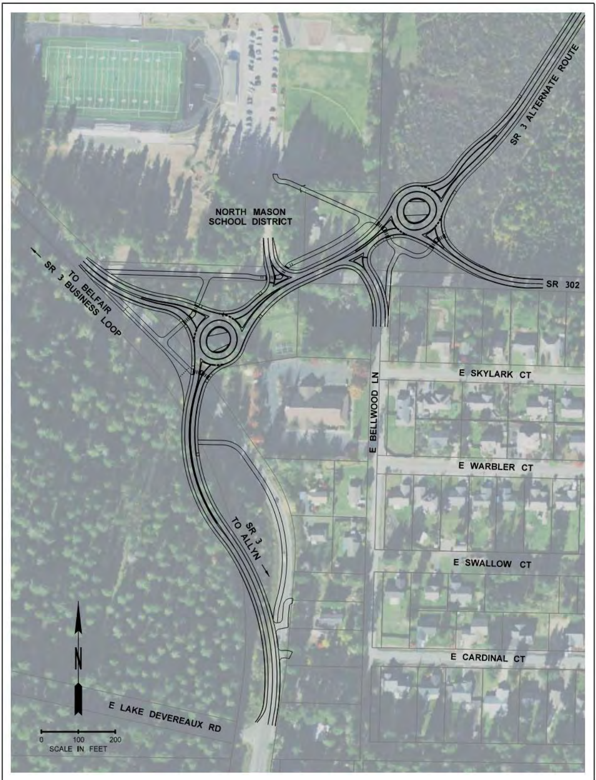
Figure 3: South End Roundabout Connections
