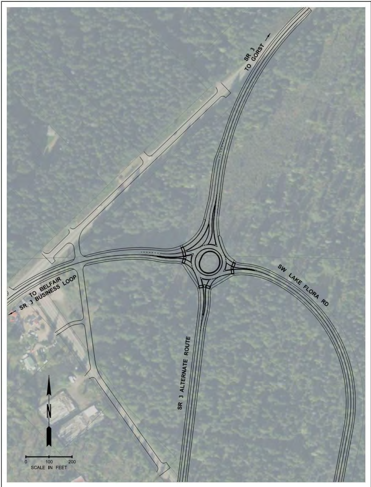
Figure 4: North End Roundabout Connection
