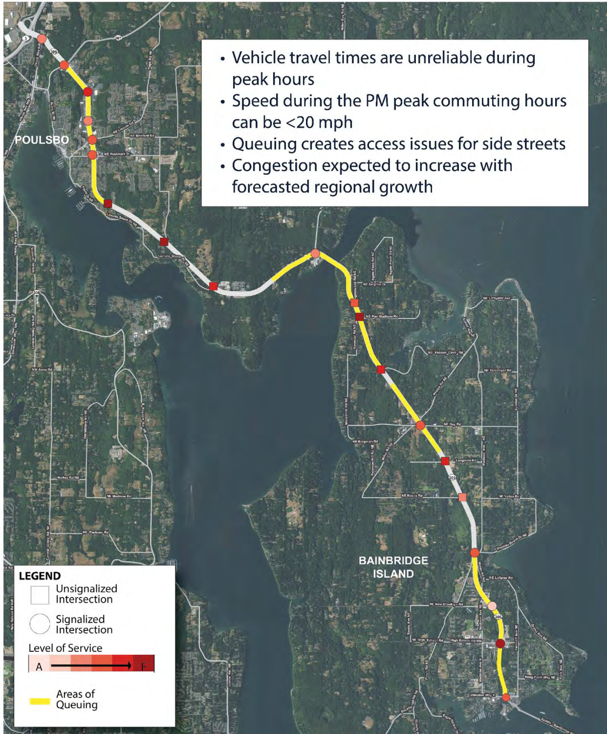
Figure 8. Existing Level of Service and Queues
