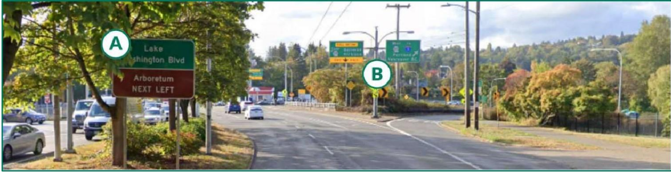
Cantilever arm: Single beam or support that extends horizontally from a fixed point without additional support underneath, allowing it to hold weight or carry loads (such as signs) at its free end. Pictured above: Cantilever arm on NE 8 th Street in Bellevue.
