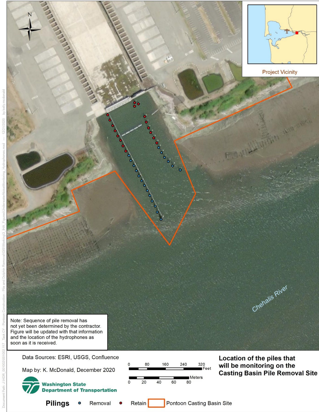
Figure 3. Location of the piles that will be monitored on the casting basin pile removal site.
