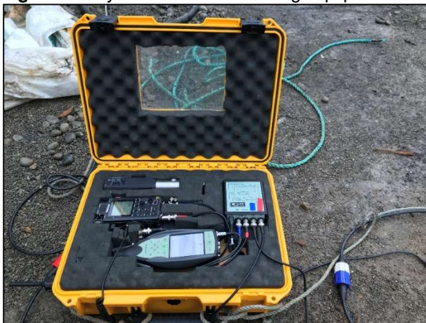
Figure 6.1 Hydroacoustic Monitoring Equipment
