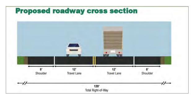
Figure 2. SR 3 Proposed Highway Cross-section
