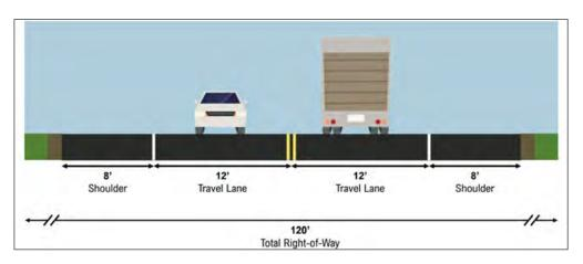
Figure 2. SR 3 Proposed Highway Cross-section
