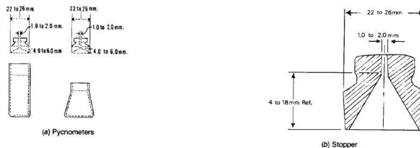
FIG. 1 Suitable Pycnometers and Stopper
