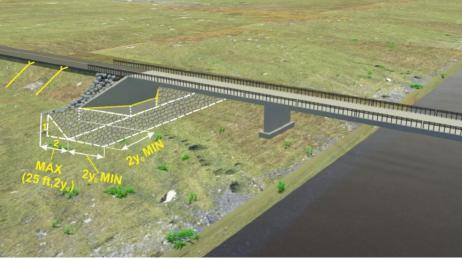
Takeaway: For crossings with abutment toes near to the main channel and/or if the crossing is likely to experience lateral migration, Scour Condition A should be used and selected in both SMS and HT.
