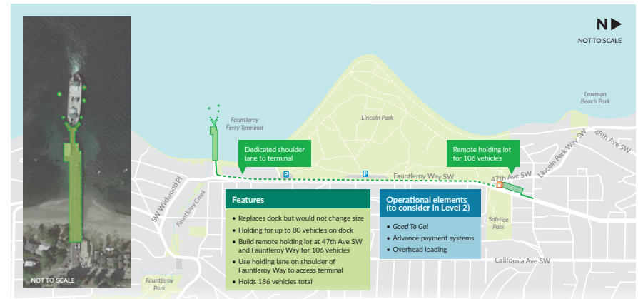
Alternative A-6: Replace dock at same size and location and add remote holding at 47th Avenue Southwest and Fautleroy Way
