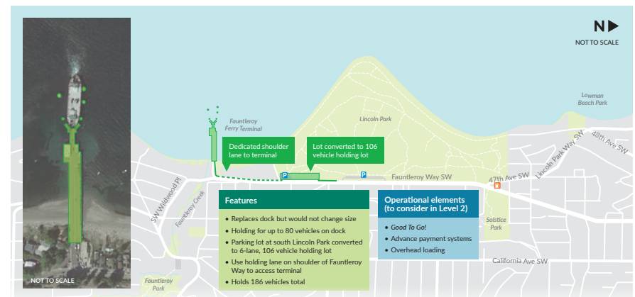
AND Alternative A-7: Replace dock at same size and location and add remote holding at Lincoln Park
