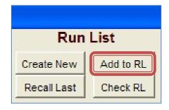
Tip: The file name will be added where the current focus is in your run-list. By default, it will be at the bottom of the list. After adding a file name, the focus automatically moved down to the next position.
