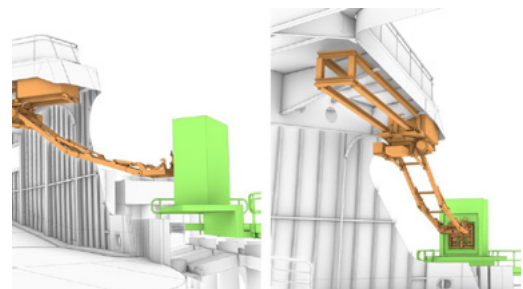
A robotic charging arm will extend from the hybrid electric ferries to the terminal power source to recharge the batteries as loading and unloading takes place.
