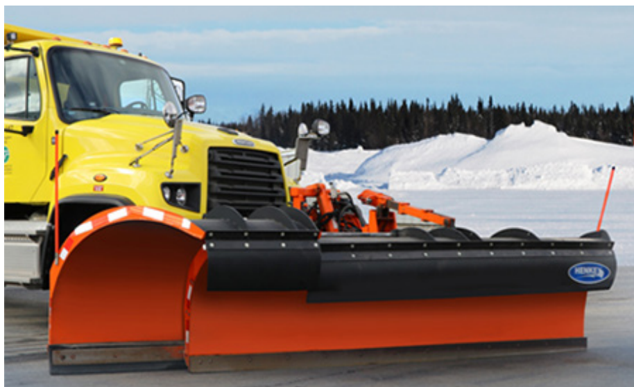
WSDOT's extended snowplow adds 3-feet of width to a standard plow and allows maintenance crews to clear snow from traveled lanes and shoulders on secondary highways with a single pass.
