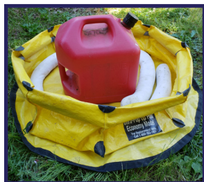
Make sure fluids and appropriate equipment are stored onsite with secondary containment.
