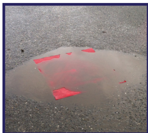
Drain seal to keep spill at the surface.
