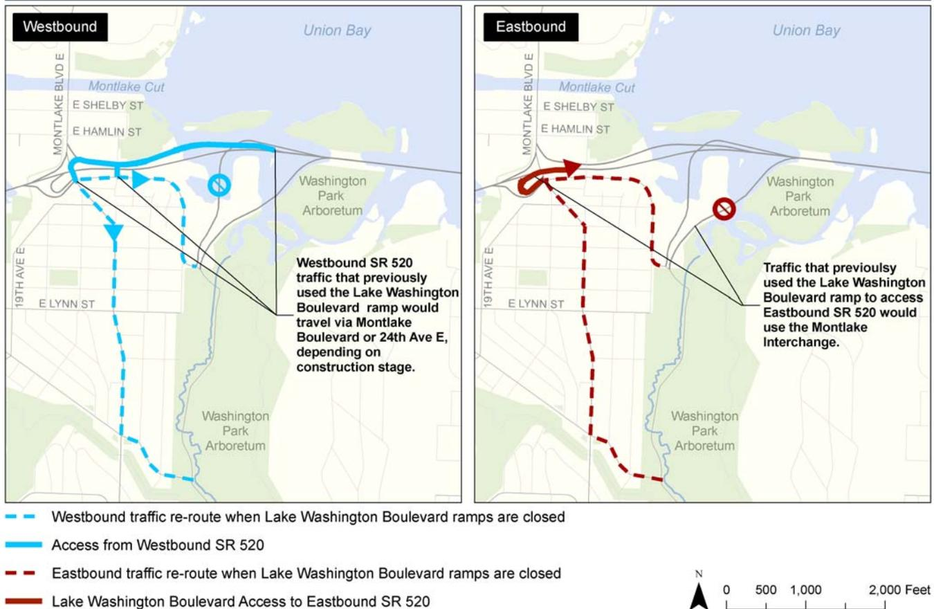
WSDOT would make several capacity improvements to the intersections on Montlake Boulevard before closing the Lake Washington Boulevard ramps. The improvements would accommodate the expected increases in traffic volumes and minimize substantial delays that otherwise would occur on Montlake Boulevard at SR 520. These improvements would help offset the effects of the Lake Washington Boulevard ramp closure. The proposed changes in the Montlake area include the following:
