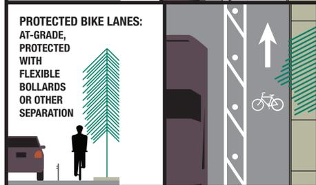
PROTECTED BIKE LANES: AT-GRADE, PROTECTED WITH FLEXIBLE BOLLARDS OR OTHER SEPARATION
