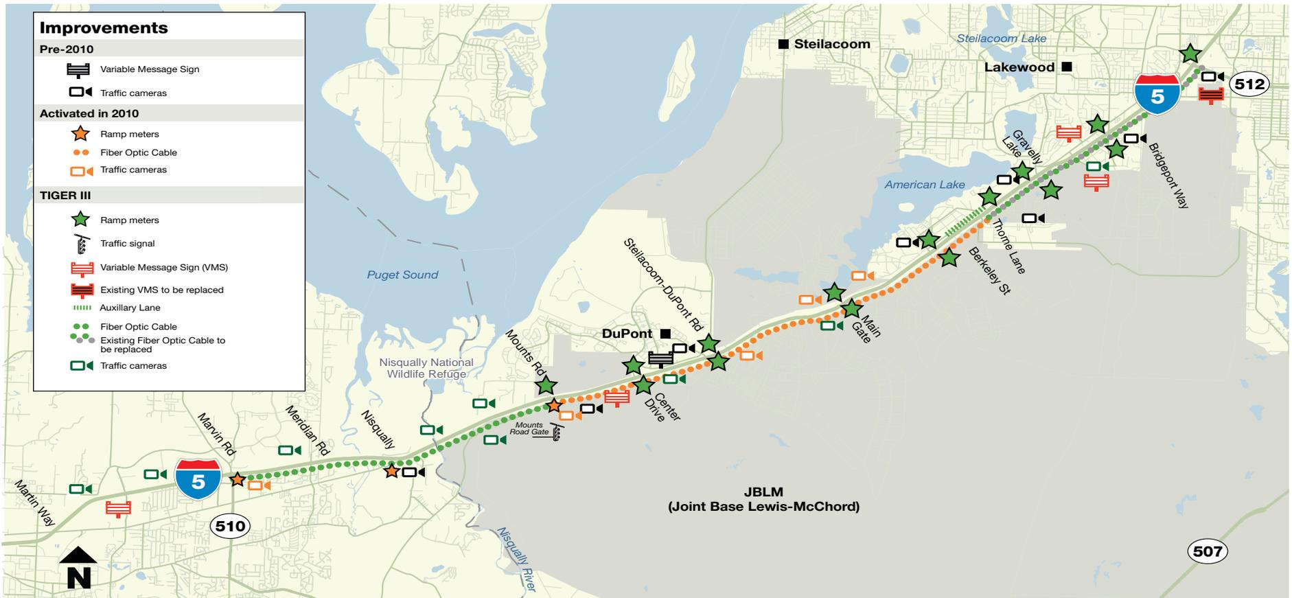
**Variable Message Signs (VMS):** A VMS is an electronic traffic sign used on roadways to provide motorists important information about traffic congestion, incidents, roadwork, travel times, special events or speed limits on a specific highway segment. They may also recommend alternative routes, limit travel speed, warn of duration and location of problem or simply provide alerts or warnings.
