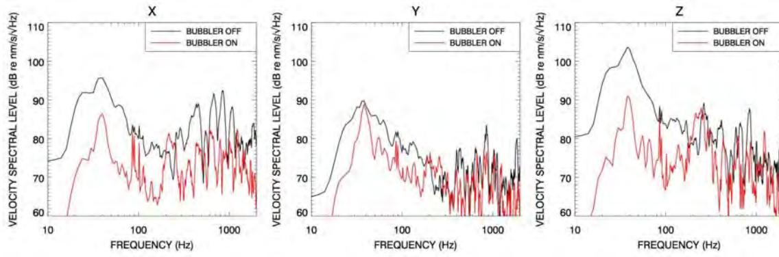
**Figure 9:** Average X, Y and Z velocity spectral levels for pile T8 impact hammering traces. The inactive bubble curtain spectra are shown in black and the active bubble curtain spectra are shown in red.
