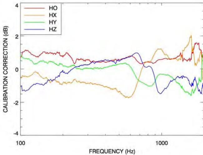
**Figure 5:** Plot of relative hydrophone sensitivity, versus frequency, as determined by cross-calibration procedure. Nominal hydrophone sensitivity is  $-201$  dB re V/ $\mu$ Pa.
