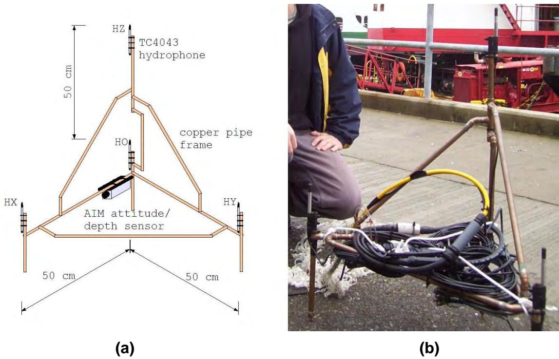
**Figure 4:** (a) Schematic diagram of the pressure gradient sensor shown in isometric projection. Four Reson TC4043 hydrophones are located at the positions indicated HO (origin) HX (x-axis) HY (y-axis) and HZ (z-axis). The AIM attitude/depth sensor is oriented in the X-direction. The axial hydrophones HX, HY and HZ are all located 50 cm from the origin hydrophone HO. (b) Photograph of the pressure gradient sensor with attached hydrophone cables.
