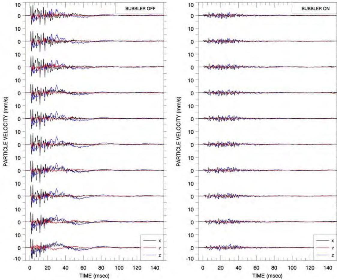
**Figure 8:** Triaxial particle velocity traces from hammering of pile T8 showing comparison between inactive bubble curtain (left) and active bubble curtain (right). Measurements were taken at 10 meters horizontal range and 5 meters depth.
