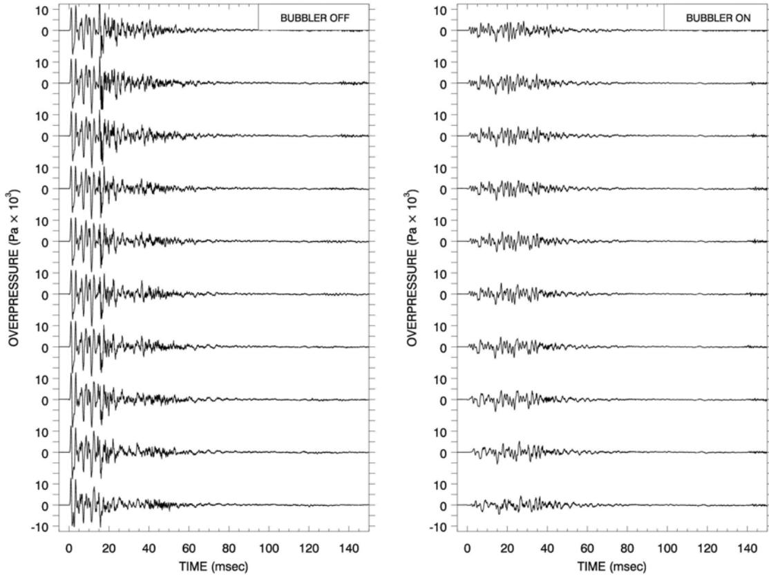
**Figure 6:** Pressure waveforms from impact hammering of pile T8 showing comparison between inactive bubble curtain (left) and active bubble curtain (right). Measurements were taken at 10 meters horizontal range and 5 meters depth.
