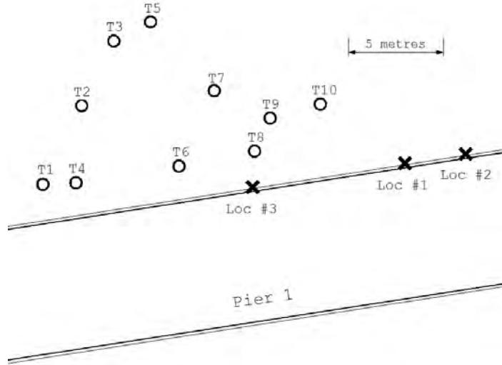
**Figure 3:** Plan view diagram of construction site showing the layout of the steel piles (labelled T1 through T10) and approximate deployment locations of the acoustic sensor (Loc #1, Loc #2 and Loc #3).
