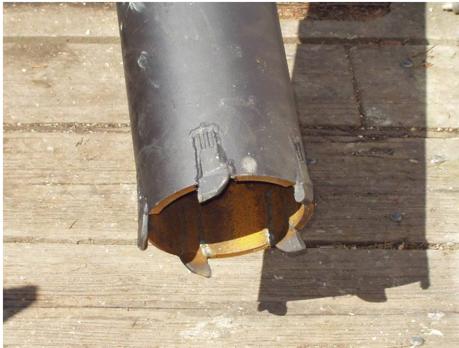
Figure 2-8 Serrated Edge of a Micropile
