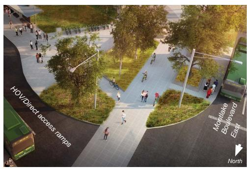
A conceptual rendering showing a bird's-eye view of the "Urban Trailhead" area of the future Montlake lid over SR 520. A continuous paving pattern extends the character of the sidewalk across the SR 520 HOV/Direct access lanes (view facing southeast).
