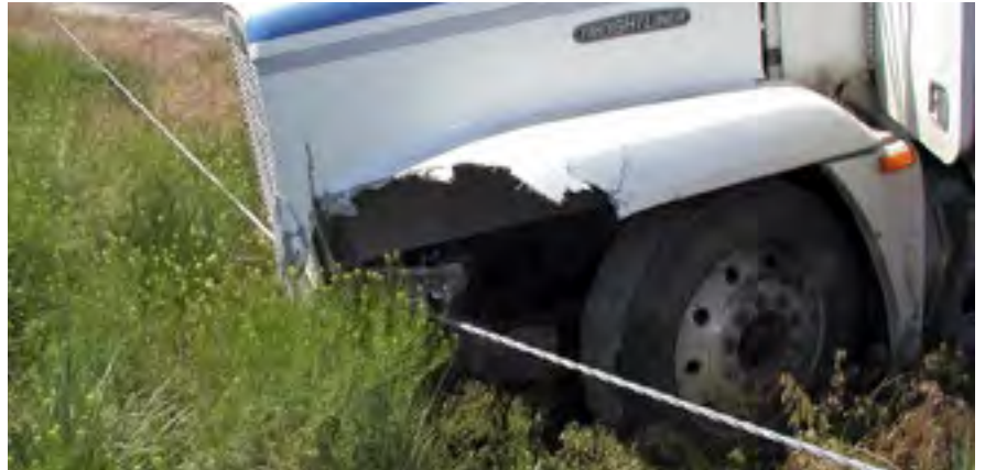
Low-cost safety strategy: cable barrier
