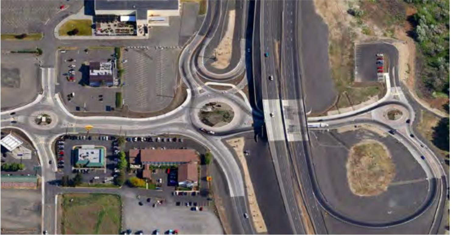
on-ramps and off-ramps to Valley Mall Boulevard and the adjacent local street, to improve traffic flow, reduce the risk of collisions and accommodate future growth. Construction on the I-82/Valley Mall Blvd interchange was complete in 2011.
