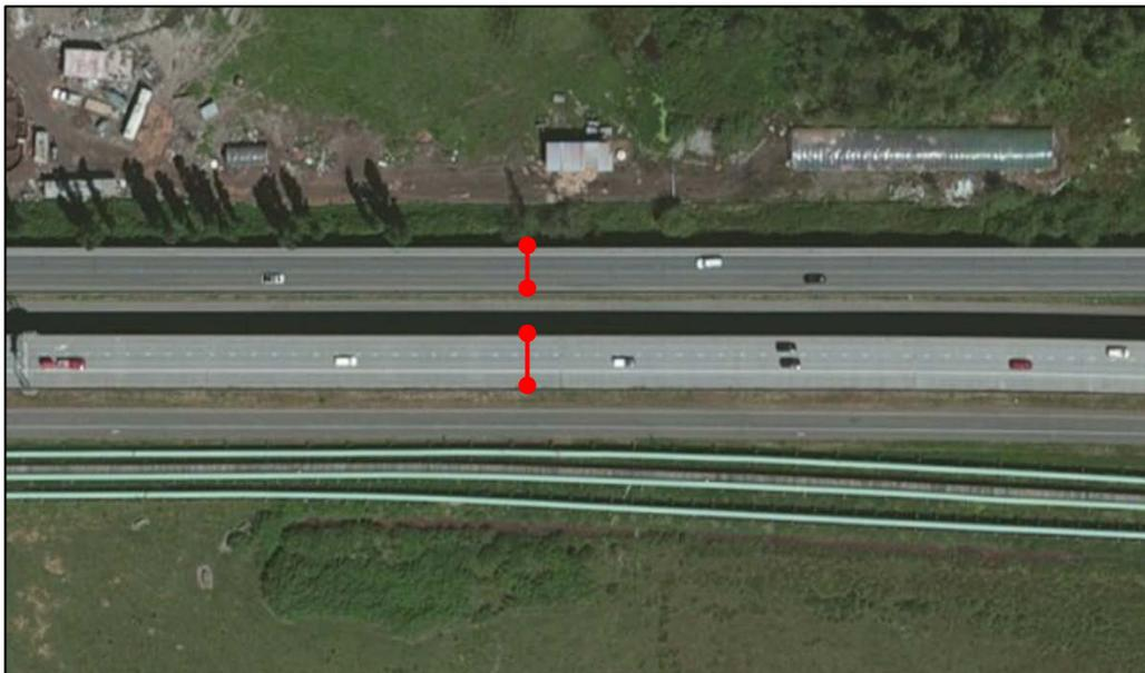
Additionally, model the outside edge of pavement close to the actual location. For example, in the upper road, the outside edge of shoulder is 14 feet from the center of the travel lanes, so a pavement width should be modeled at 28 feet. The lower road outside edge of shoulder is 19 feet from the center of the travel lanes, so a 38 foot pavement width should be modeled.
