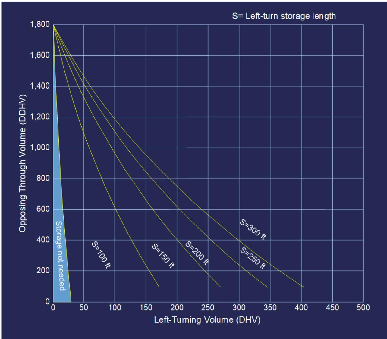
Determine the storage length on two-lane highways by using [Exhibit 1310-11](#) through [Exhibit 1310-13](#). On four-lane highways, use [Exhibit 1310-10](#). These lengths do not consider trucks. Use [Exhibit 1310-14](#) for storage length when trucks are present.
