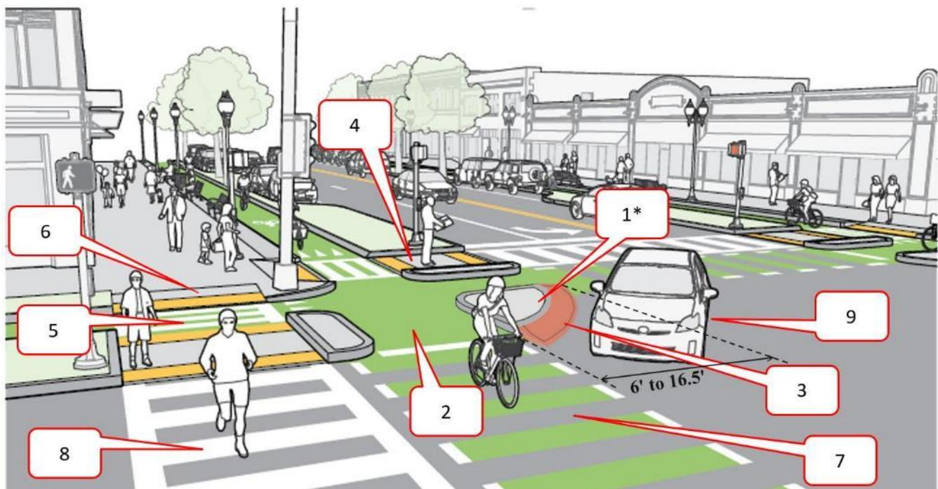
1. Corner island minimizes the right-turn radius - this defines a path that encourages a lower vehicle turning speed (see Section 1510.09(6))
