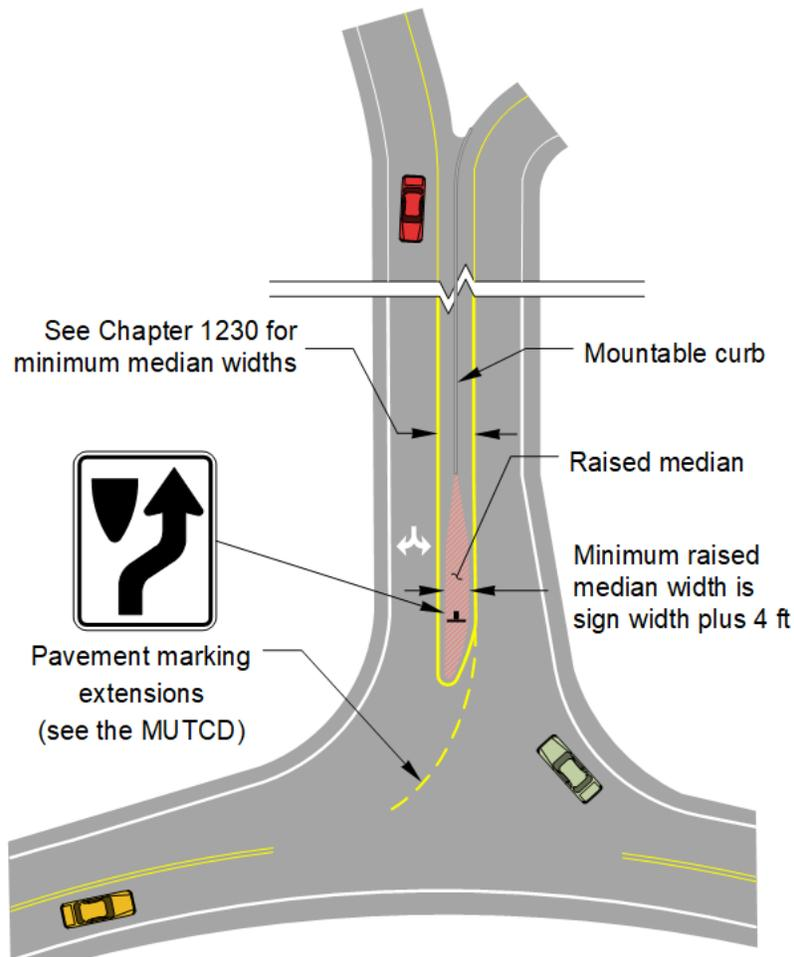
**b. Reduced Off-Ramp Terminal Throat Width**
