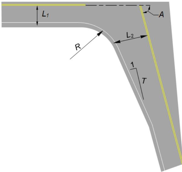
$L_1$  = Available roadway width [2] that the vehicle is turning from
