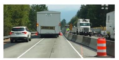
Oversized truck freight example; modular home straddling both lanes on Interstate 90 at a bridge rehabilitation work zone with a reduced traveled way.
