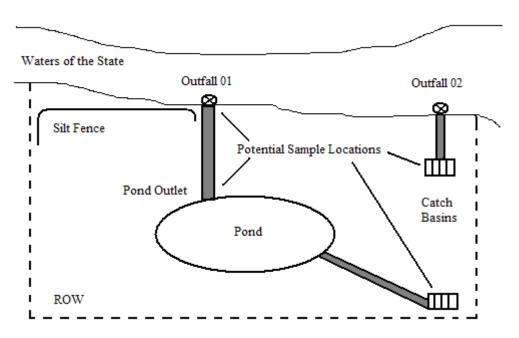
Figure 6-5.1 General layout of NPDES Construction Stormwater General Permit water quality sampling locations.
