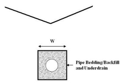
Figure RT.07.4 Media filter drain underdrain installation.
