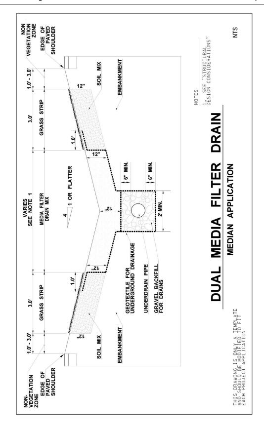
Figure RT.07.2 Dual media filter drain: Median application.
