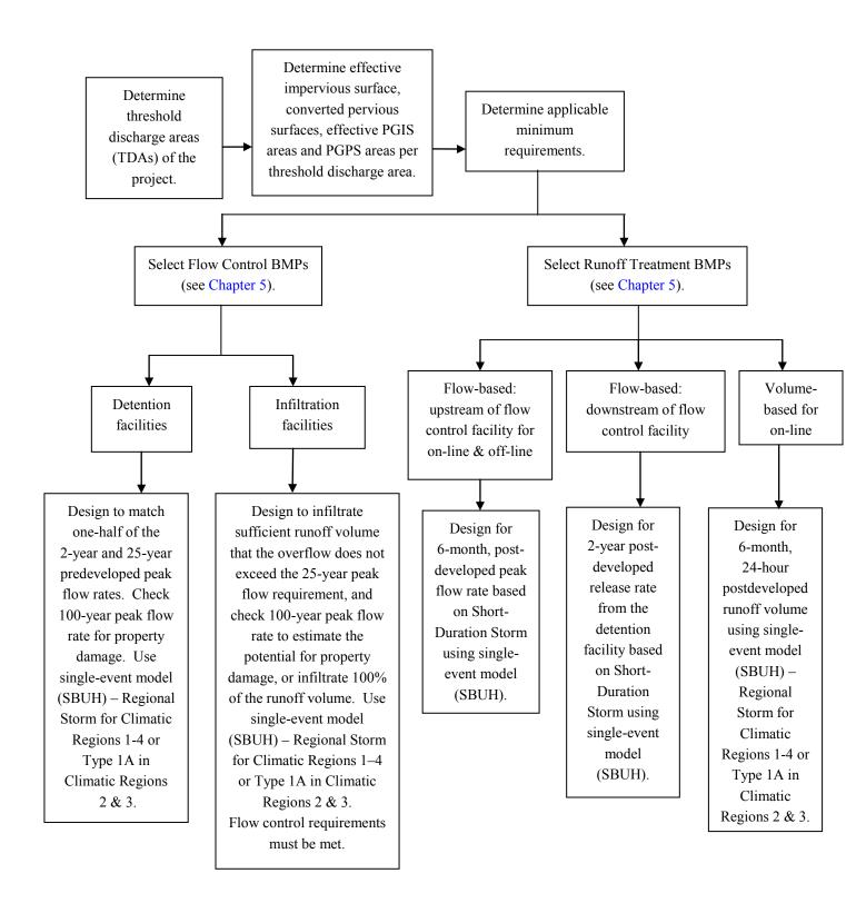
Figure 4-5 Hydrologic analysis flowchart for eastern Washington.
