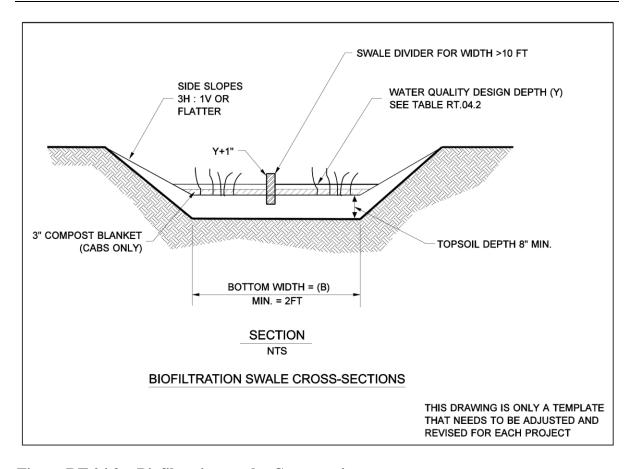
Figure RT.04.2 Biofiltration swale: Cross section.
