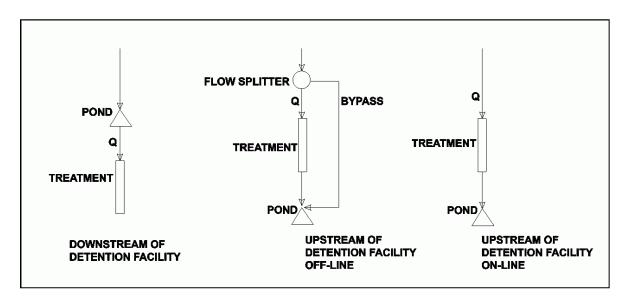
Figure 4-6 Typical on-line and off-line facility configurations.
