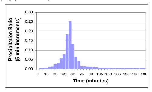
Figure 4C-3 Short-duration storm unit hyetograph.
