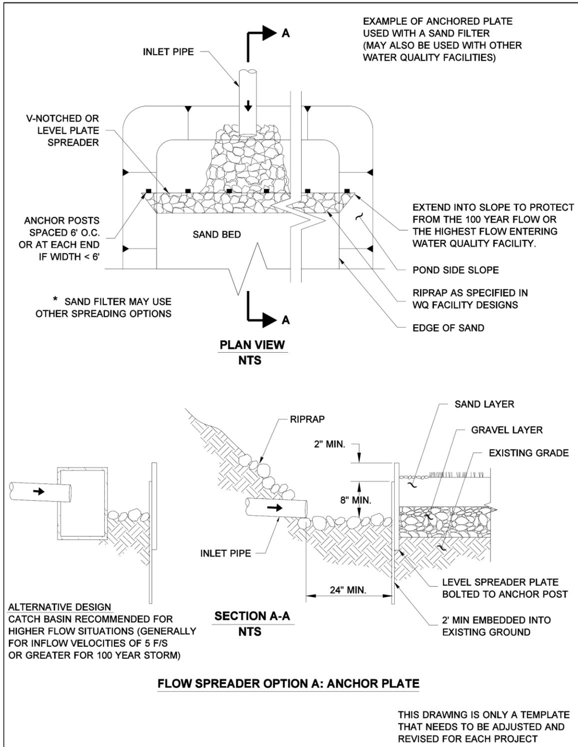
Figure 5.4.3.4 Flow spreader Option A: Anchor plate.
