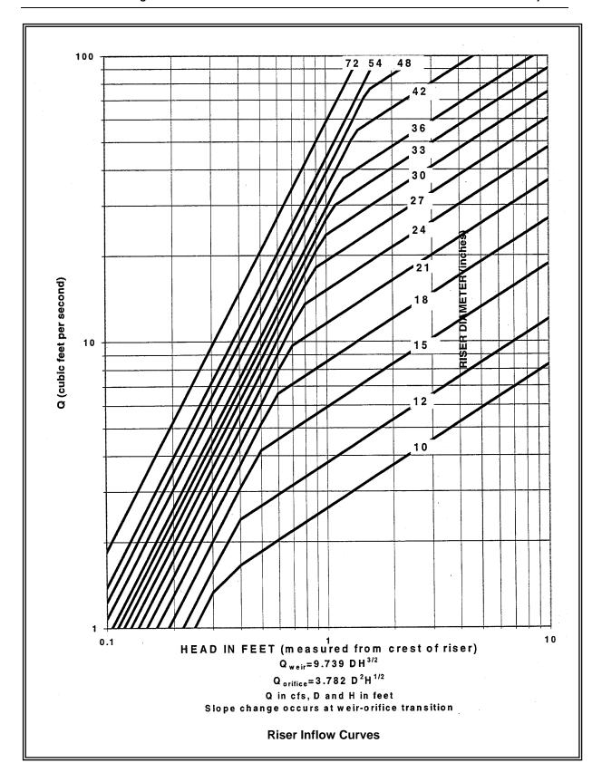
Figure FC.03.5 Overflow structure sizing.
