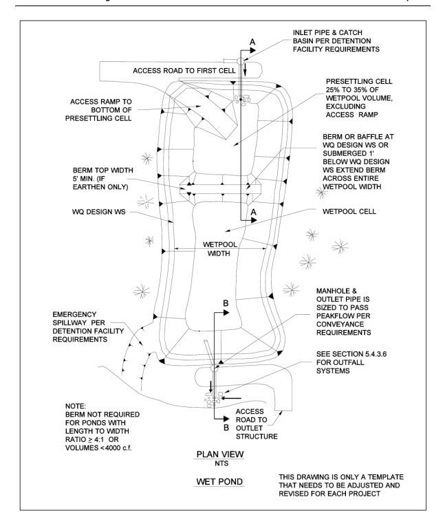
Figure RT.12.1 Wet pond: Plan view.
