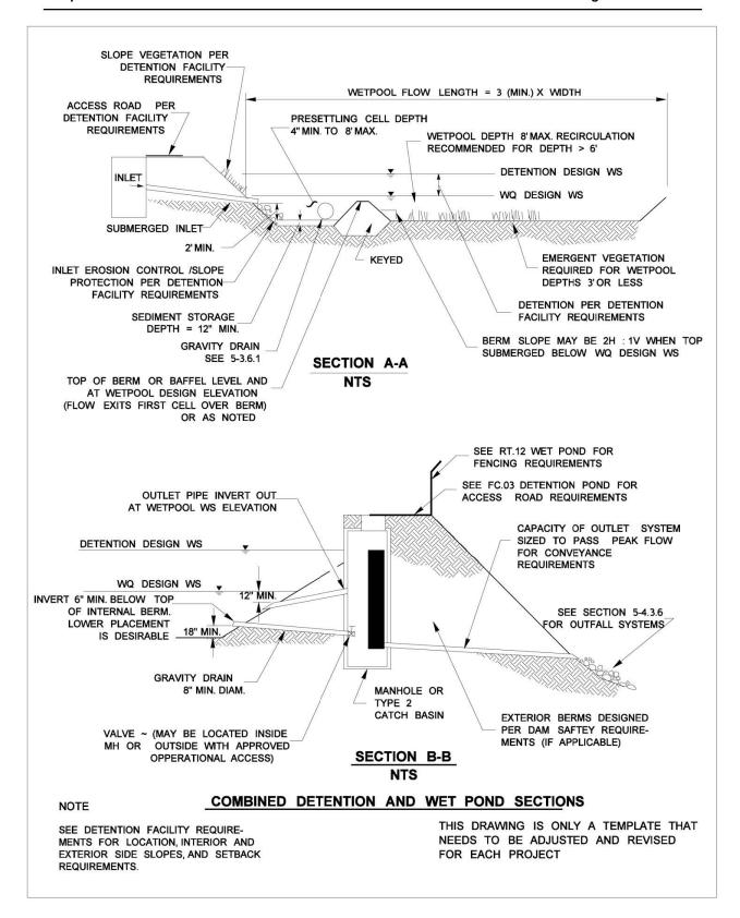
Figure CO.01.2 Combined detention and wet pond: Cross sections.
