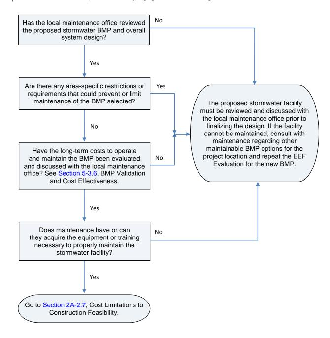
Figure 2A-5 Maintenance limitations to construction feasibility.
