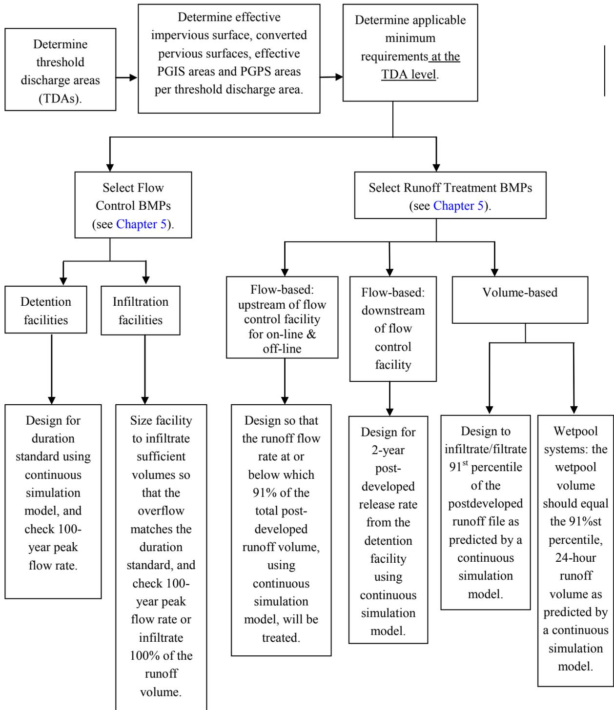
Figure 4-4 Hydrologic analysis flowchart for western Washington.
