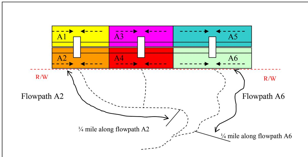
Figure 4-2b Threshold discharge areas (plan – not to scale).
