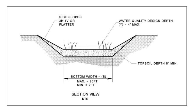
Figure RT.05.1 Wet biofiltration swale: Cross section.
