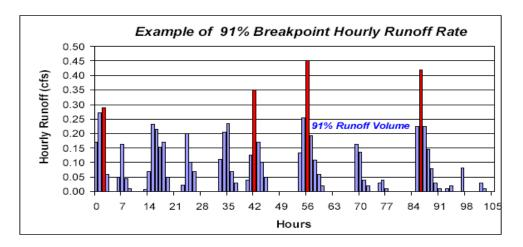
Figure 4-8 Example showing calculation of runoff treatment discharge for on-line treatment facilities—computed as 0.28cfs.
