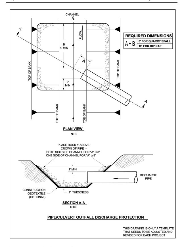
Figure 5.4.3.8 Pipe/culvert outfall discharge.
