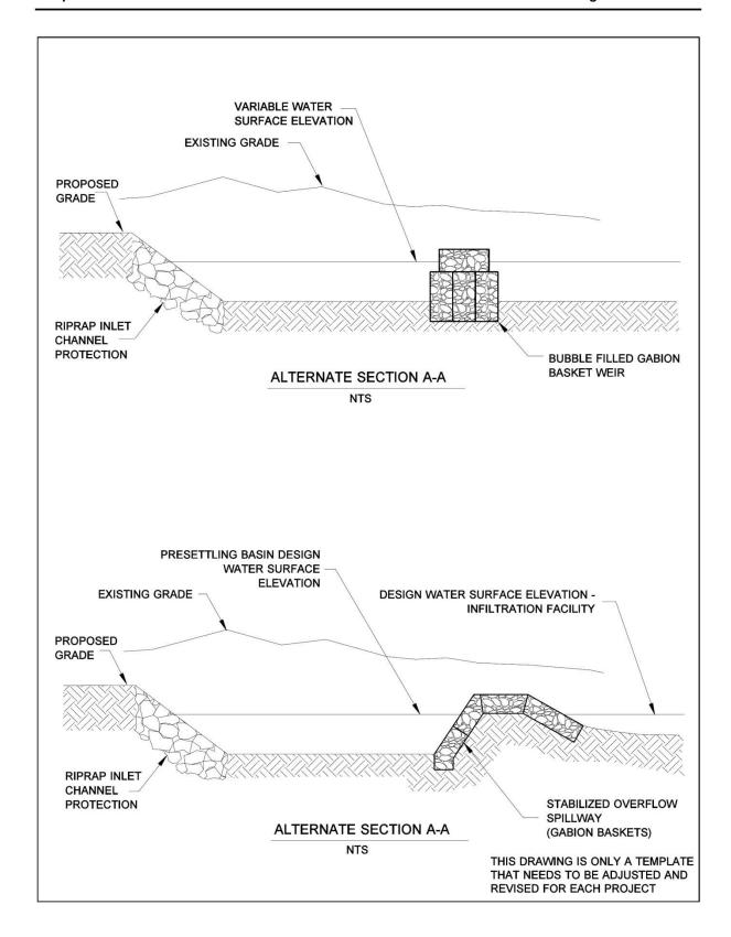
Figure RT.24.2 Presettling/sedimentation basin: Alternate sections.
