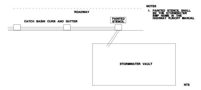
Figure 5.4.3.17 Signing for underground-type BMPs.
