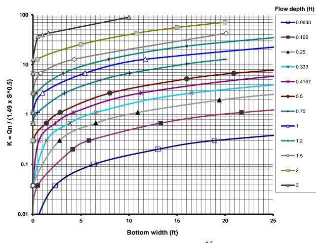
Figure RT.04.6 Open channel flow parameter,  $Qn/(1.49~s^{0.5})$ , versus bottom width (b) at different flow depths (z = 3).
