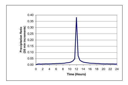
Figure 4C-2 SCS Type II hyetograph.
