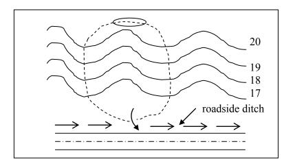
Figure 4-1 Drainage basin delineation example.
