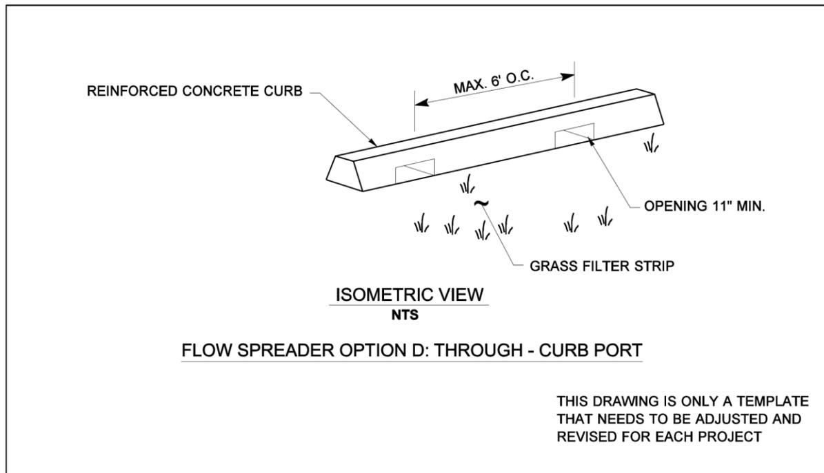
**Figure 5.4.3.7 Flow spreader Option D: Through-curb port.**
