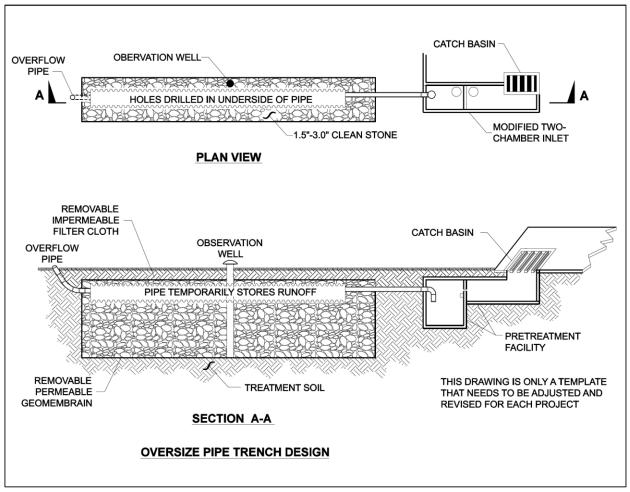
Figure IN.03.4 Oversize pipe trench design.
