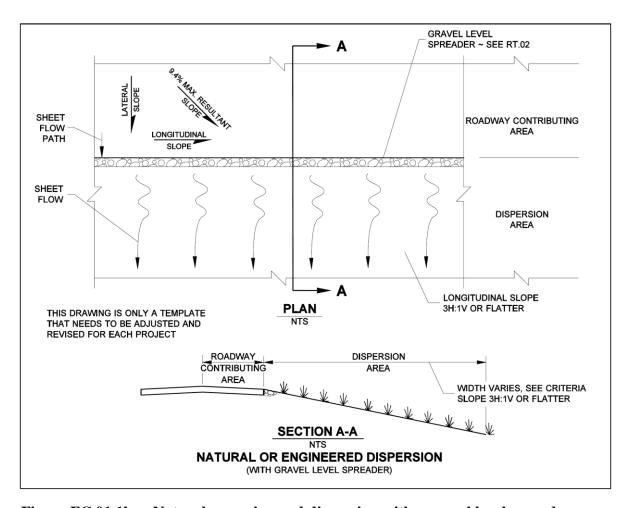
Figure FC.01.1b Natural or engineered dispersion with a gravel level spreader.
