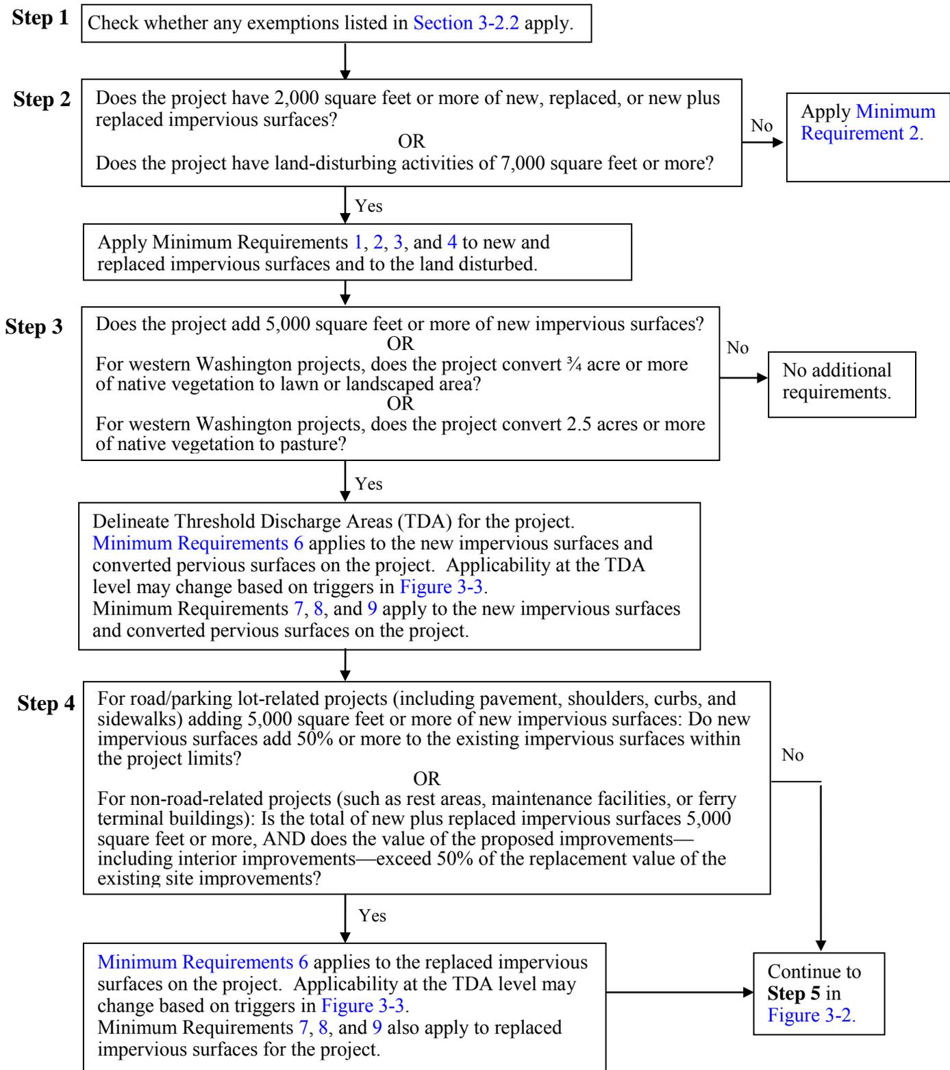
Figure 3-1 Minimum requirement applicability at project level.
