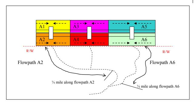
Figure 4-2b Threshold discharge areas (plan – not to scale).
