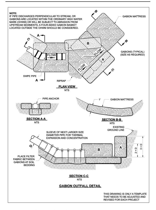
Figure 5.4.3.11 Gabion outfall detail.
