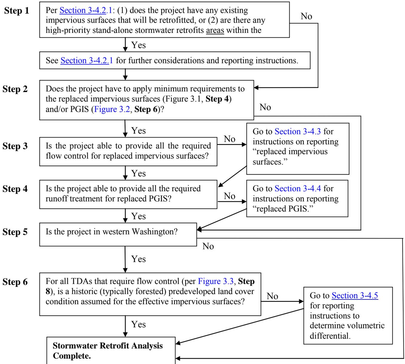
Figure 3-5 Stormwater retrofit process for WSDOT projects outside of the Puget Sound basin.
