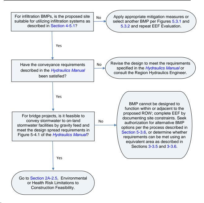
Figure 2A-3 Hydraulic limitations to construction feasibility.
