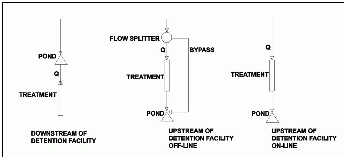
Figure 4-6 Typical on-line and off-line facility configurations.
