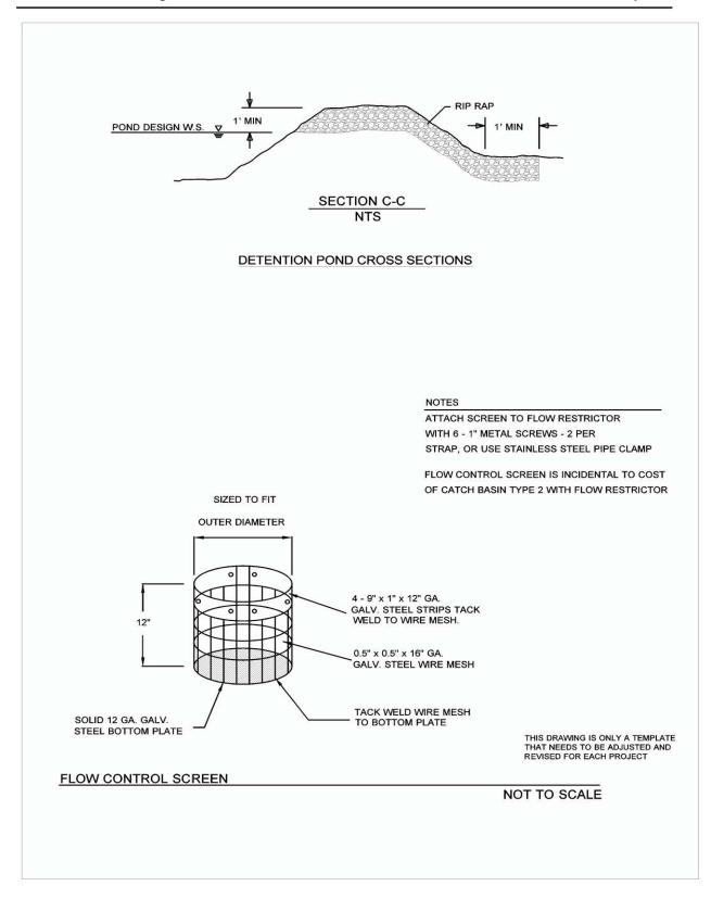
Figure FC.03.3 Detention pond: Cross sections.
