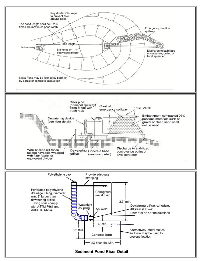
Figure 6A-1 Temporary sediment pond details.
