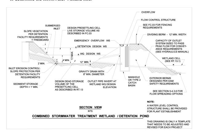
Figure CO.02.1 Combined stormwater treatment wetland/detention pond.
