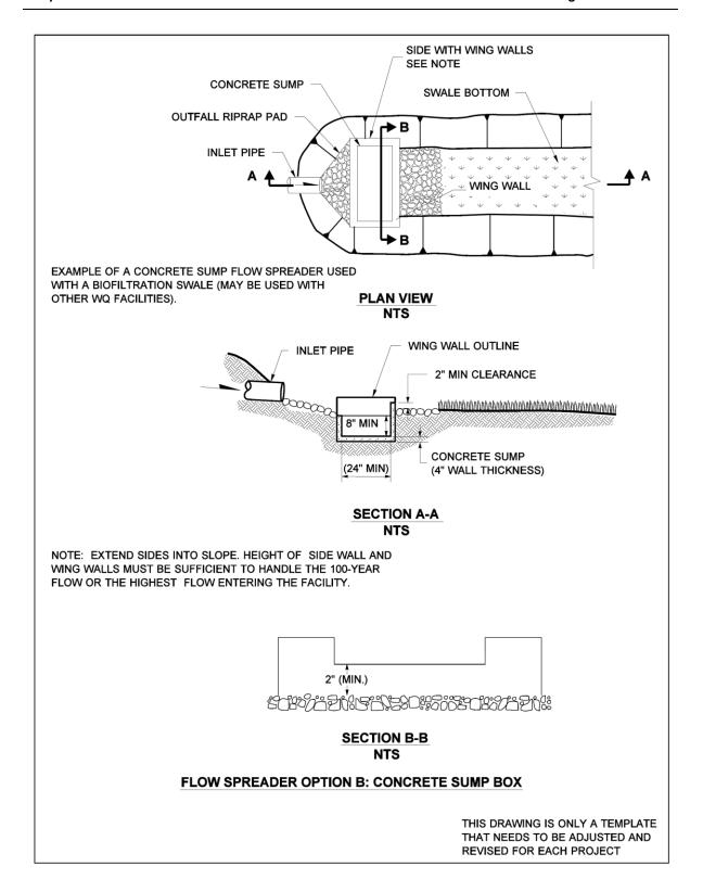
Figure 5.4.3.5 Flow spreader Option B: Concrete sump box.
