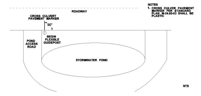
Figure 5.4.3.16 Signing for pond-type BMPs.
