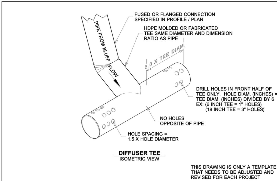
**Figure 5.4.3.12 Diffuser tee: Example of energy-dissipating end feature.**
