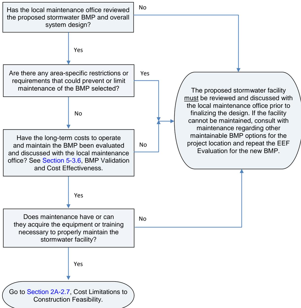
**Figure 2A-5** Maintenance limitations to construction feasibility.
