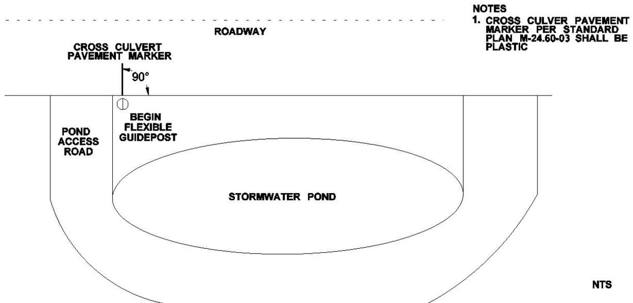
**Figure 5.4.3.16 Signing for pond-type BMPs.**
