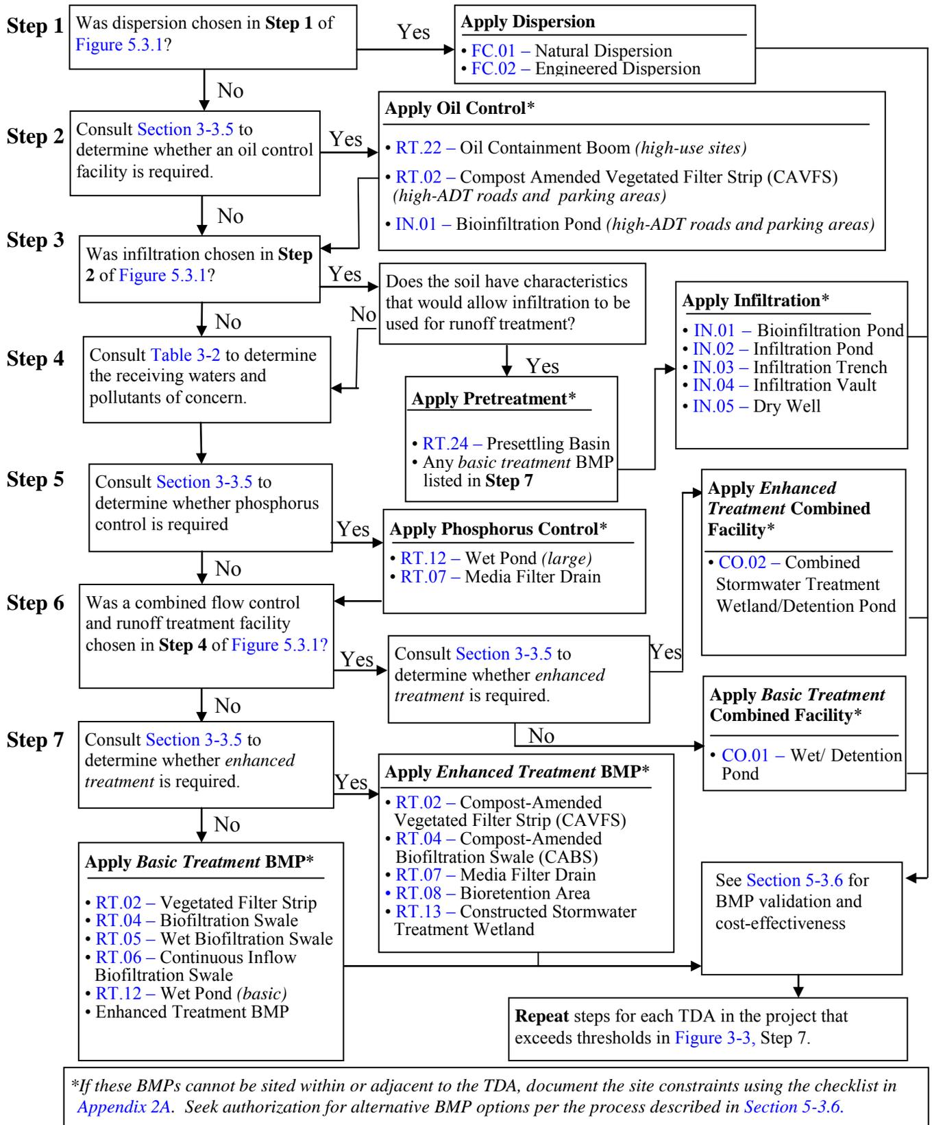
Figure 5.3.2 Runoff treatment BMP selection flow chart.
