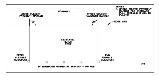
Figure 5.4.3.14 Signing for sheet flow BMPs.
