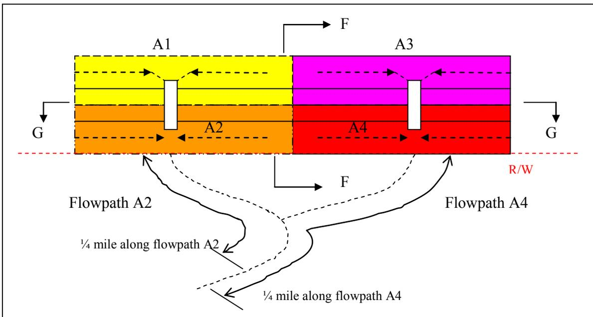
**Figure 4-2a Threshold discharge areas (plan – not to scale).**
