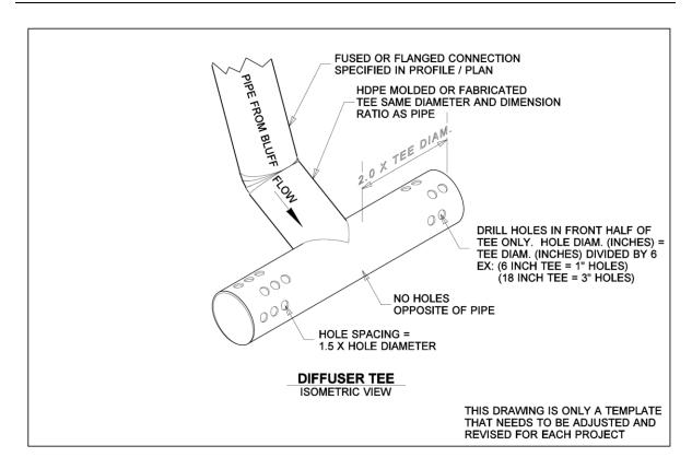
Figure 5.4.3.12 Diffuser tee: Example of energy-dissipating end feature.
