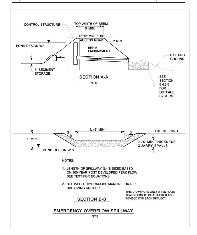
Figure FC.03.2 Detention pond: Cross sections.
