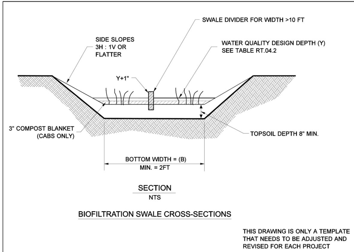
**Figure RT.04.2 Biofiltration swale: Cross section.**
