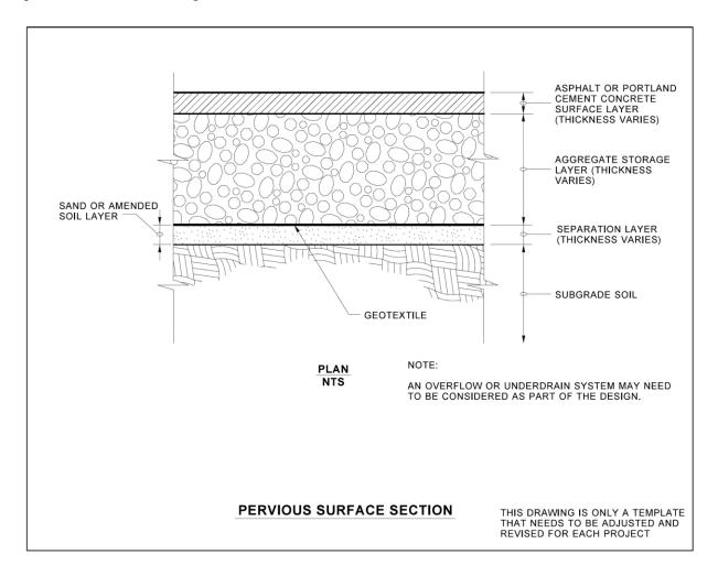
Figure IN.06.1 Permeable pavement structure elements.
