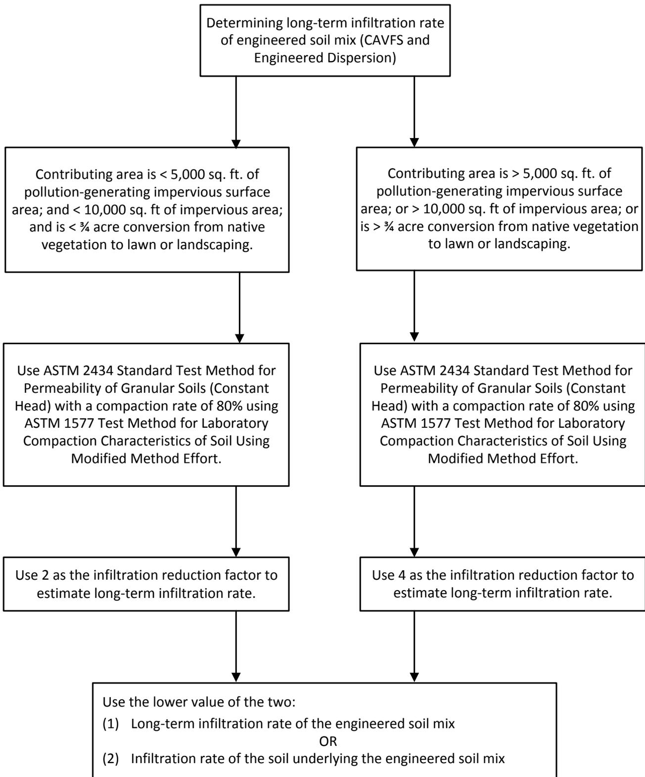
**Figure 4-16. Determining infiltration rate of soil amendments.**
