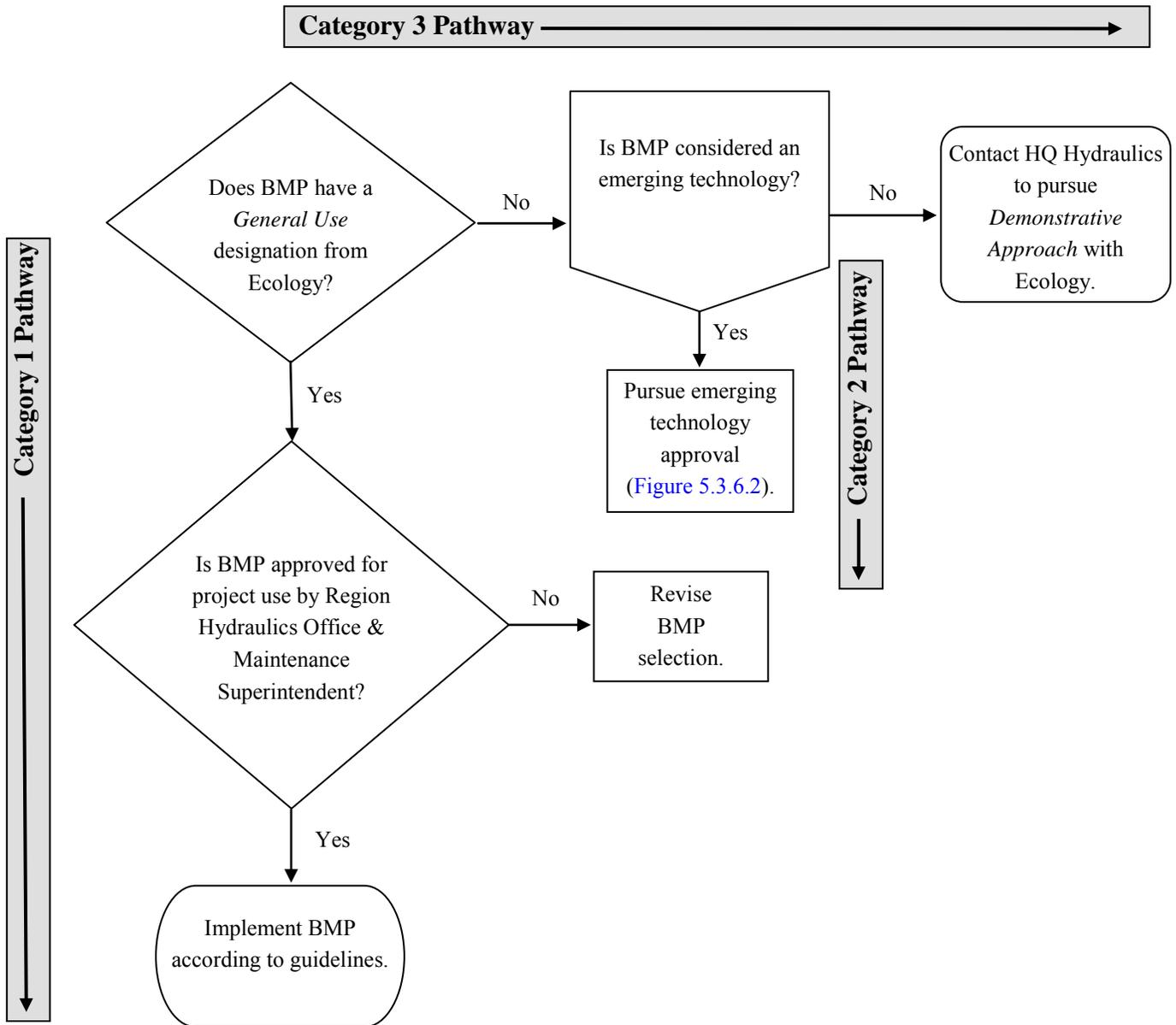
Figure 5.3.6.1 Process for using BMPs not in the HRM.
