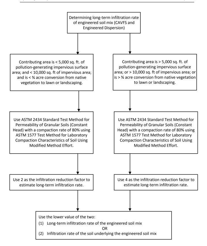
Figure 4-16. Determining infiltration rate of soil amendments.
