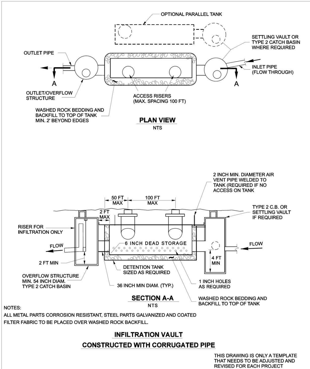
Figure IN.04.1 Infiltration vault constructed with corrugated pipe.
