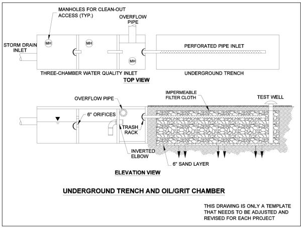
Figure IN.03.5 Underground trench and oil/grit chamber.
