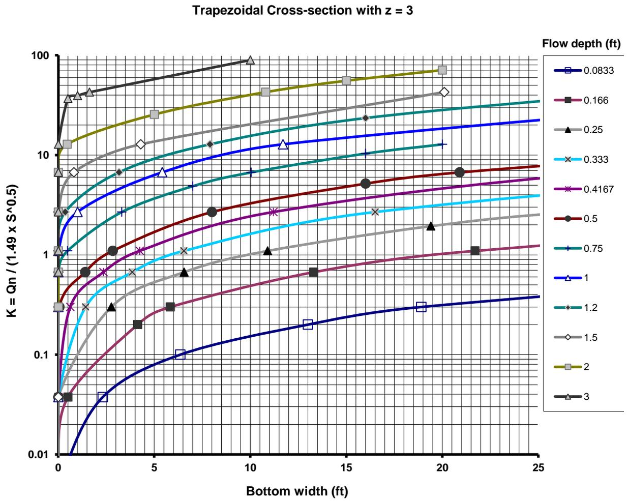
**Figure RT.04.6** Open channel flow parameter,  $Qn/(1.49 s^{0.5})$ , versus bottom width ( $b$ ) at different flow depths ( $z = 3$ ).
