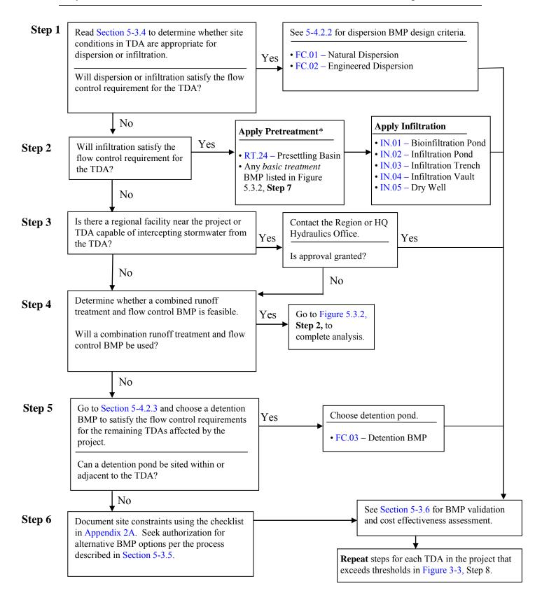
Figure 5.3.1 Flow control BMP selection flow chart.
