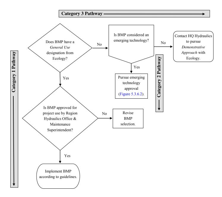
Figure 5.3.6.1 Process for using BMPs not in the HRM.
