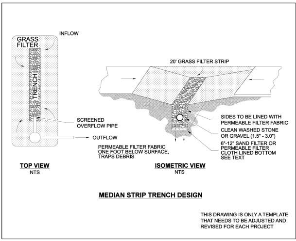
Figure IN.03.3 Median strip trench design.
