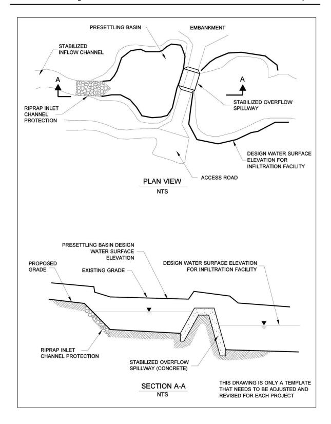
Figure RT.24.1 Typical presettling/sedimentation basin.
