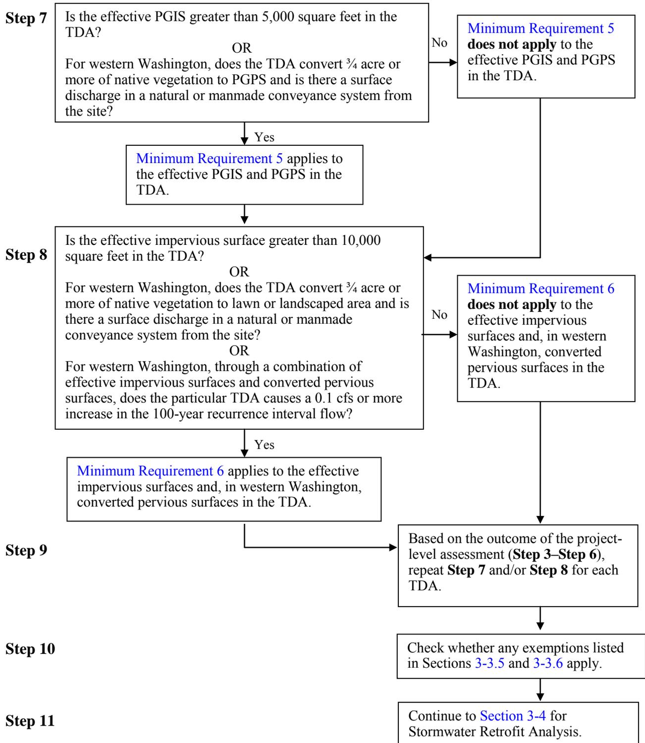
Note: For Figure 3-3, Minimum Requirements 1–4 and 7–9 still apply to all TDAs on the project, even though Minimum Requirements 5 and/or 6 may not apply to each TDA.
