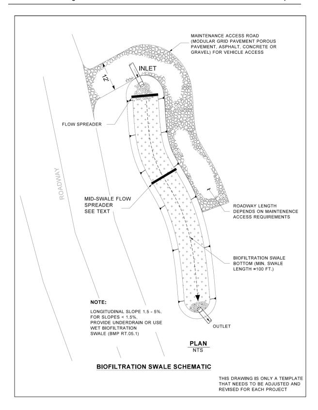
Figure RT.04.1 Biofiltration swale: Plan view.
