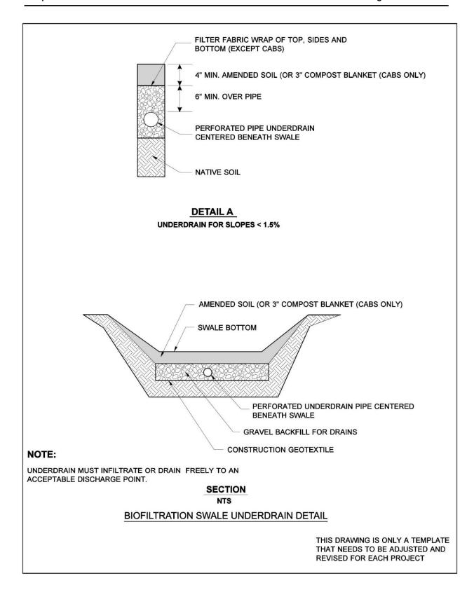
Figure RT.04.3 Biofiltration swale: Underdrain detail.
