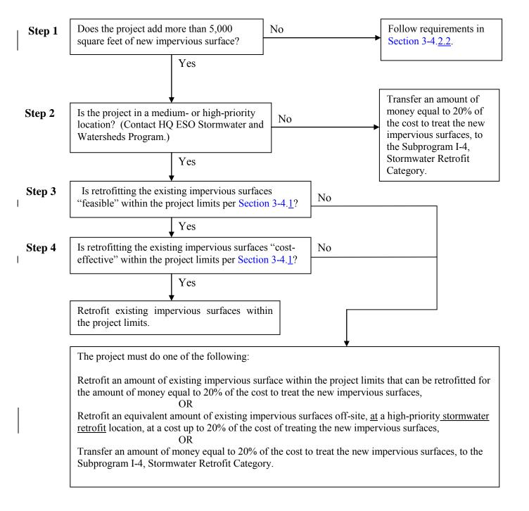
Figure 3-4 Stormwater retrofit process for WSDOT projects within the Puget Sound basin.
