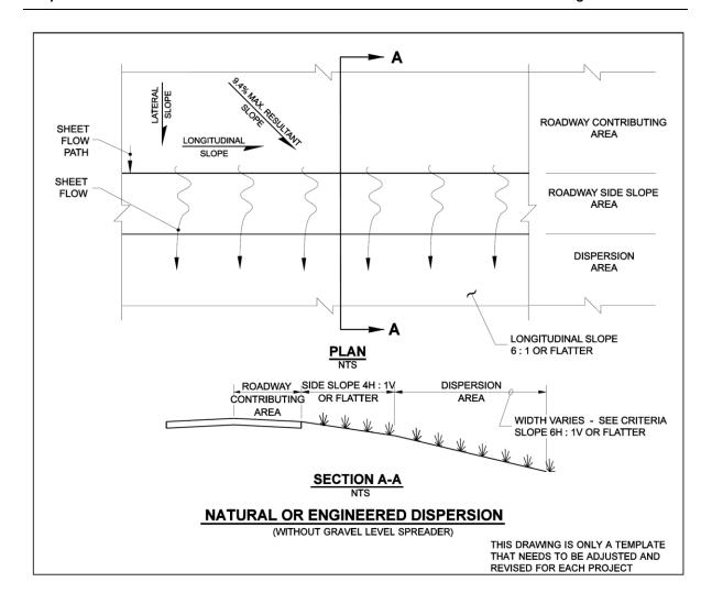
Figure FC.01.1a Natural or engineered dispersion without a gravel level spreader.
