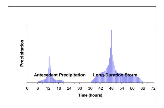
Figure 4C-4 Sample long-duration storm hyetograph.
