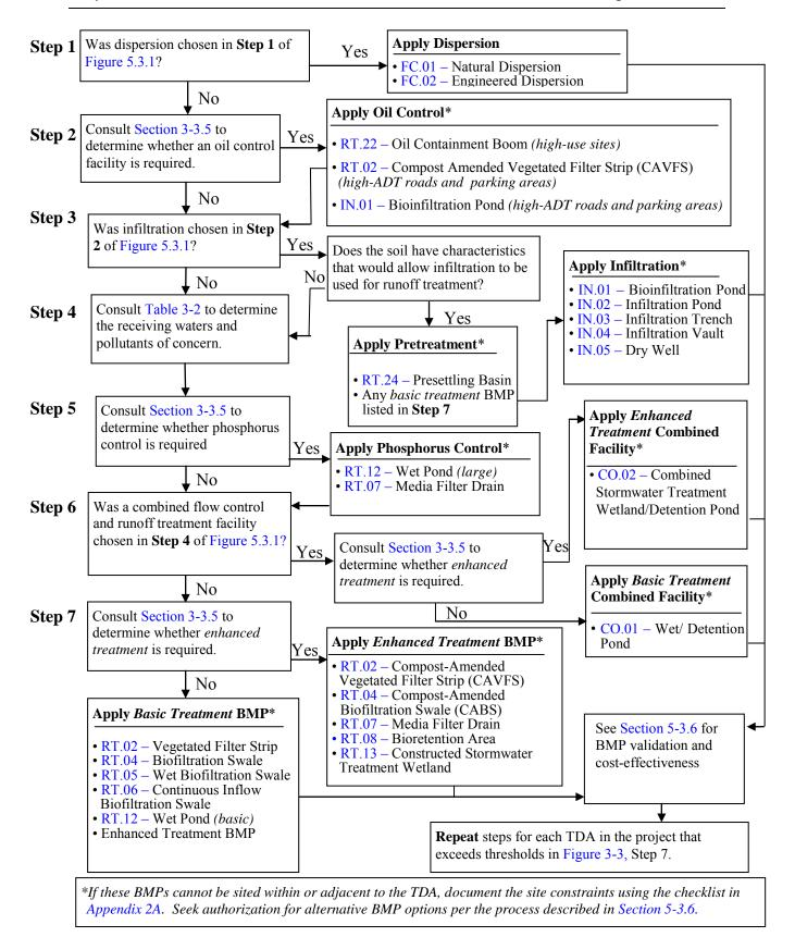
Figure 5.3.2 Runoff treatment BMP selection flow chart.
