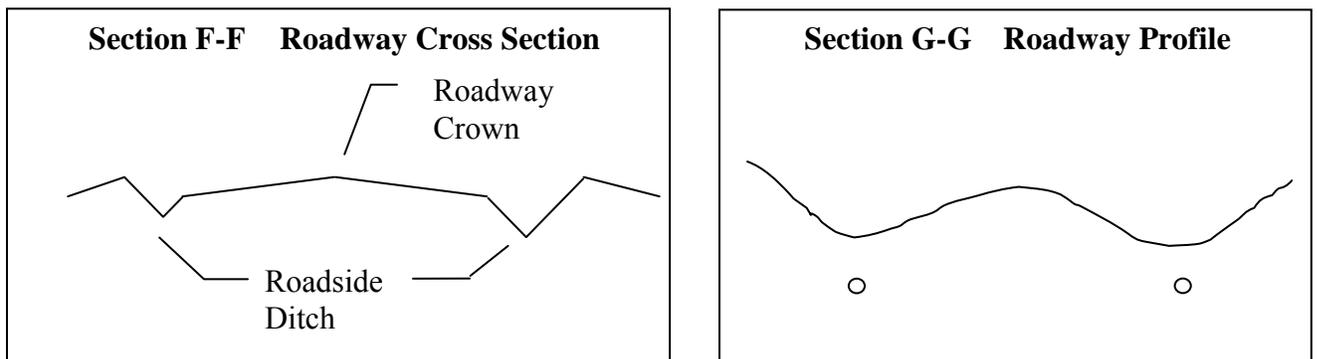
Figure 4-3 Threshold discharge areas (section and profile).
