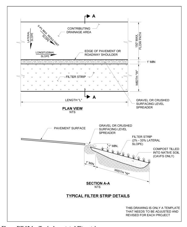
Figure RT.02.1 Typical vegetated filter strip.
