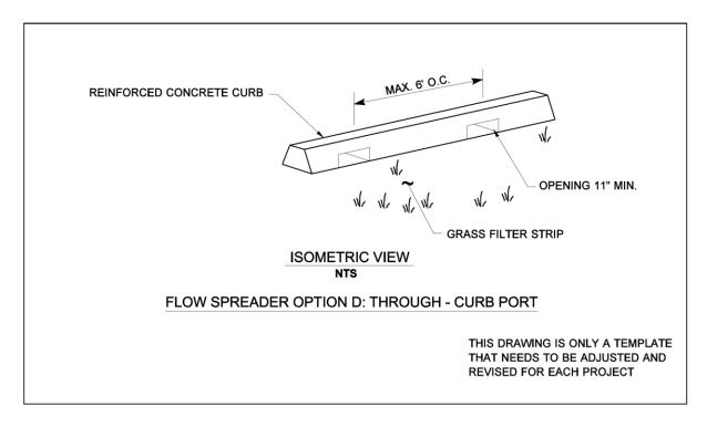
Figure 5.4.3.7 Flow spreader Option D: Through-curb port.
