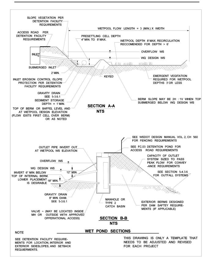
Figure RT.12.2 Wet pond: Cross section.
