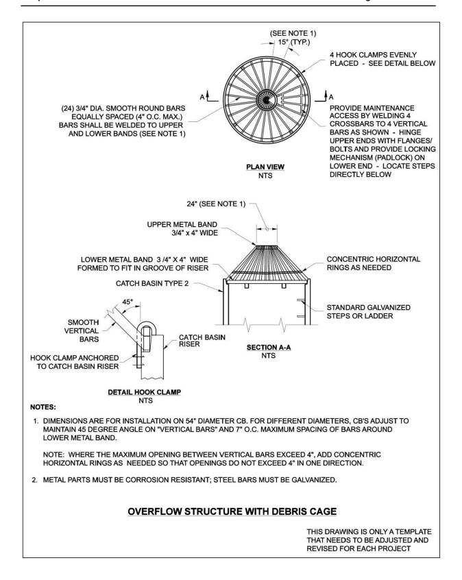
Figure FC.03.4 Overflow structure with debris cage.
