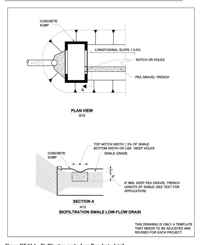
Figure RT.04.4 Biofiltration swale: Low-flow drain detail.
