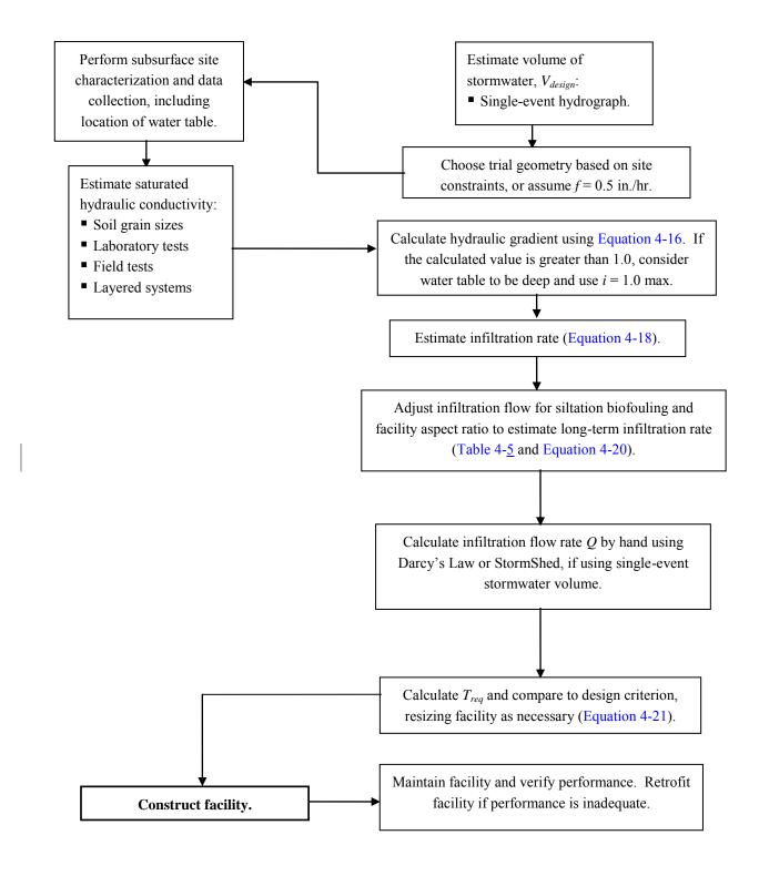
Figure 4-13 Engineering design steps for final design of infiltration facilities using the single-event hydrograph method (eastern Washington).
