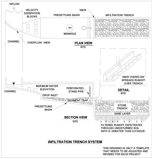
Figure IN.03.2 Infiltration trench system.
