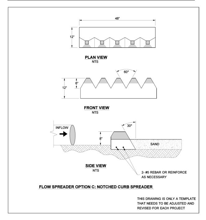
Figure 5.4.3.6 Flow spreader Option C: Notched curb spreader.
