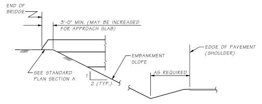
For the general case of bridges on wall type abutments or "closed" abutments, the controlling factors are the required horizontal clearance and the size of the abutment. This situation would most likely occur in an urban setting or where right of way or span length is limited.
