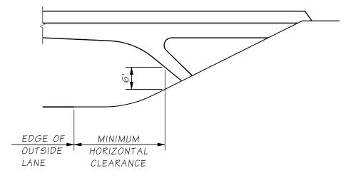
Figure 2.3.1-2 Bridge Pier in Narrow Median
