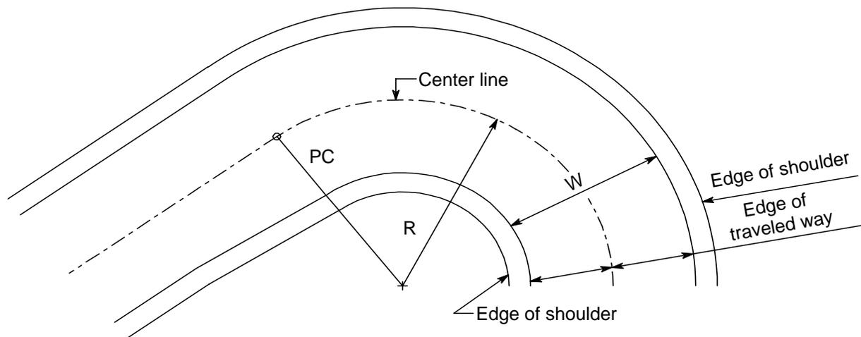
**Traveled Way Width for Two-Way Two-Lane Turning Roadways**
