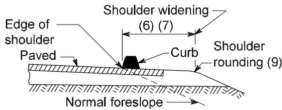
**Asphalt Concrete Curb Placement**
