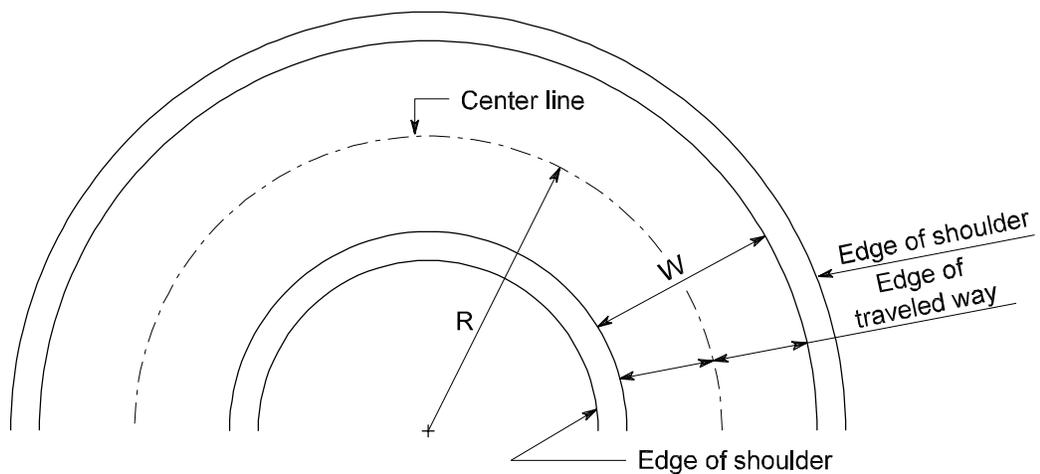
**Traveled Way Width for Two-Lane One-Way Turning Roadways**
