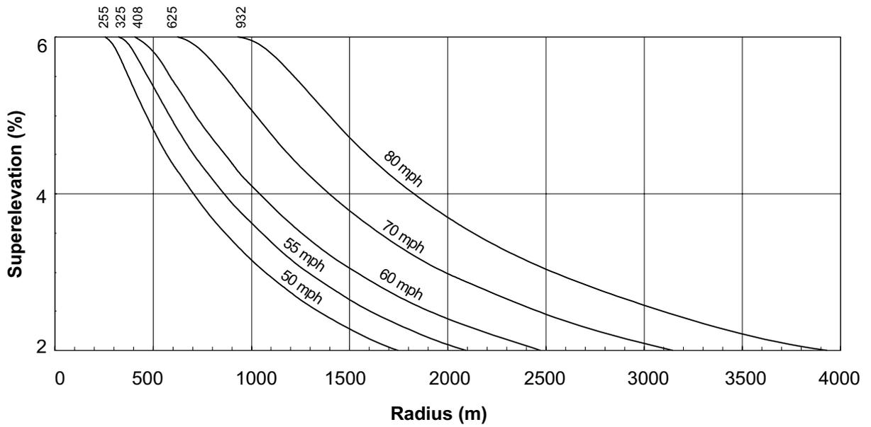
**Superelevation Rates (6% max)**
