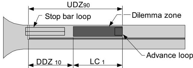
$$UDZ_{90} = \frac{V_{90}^2}{16} + V_{90}$$
