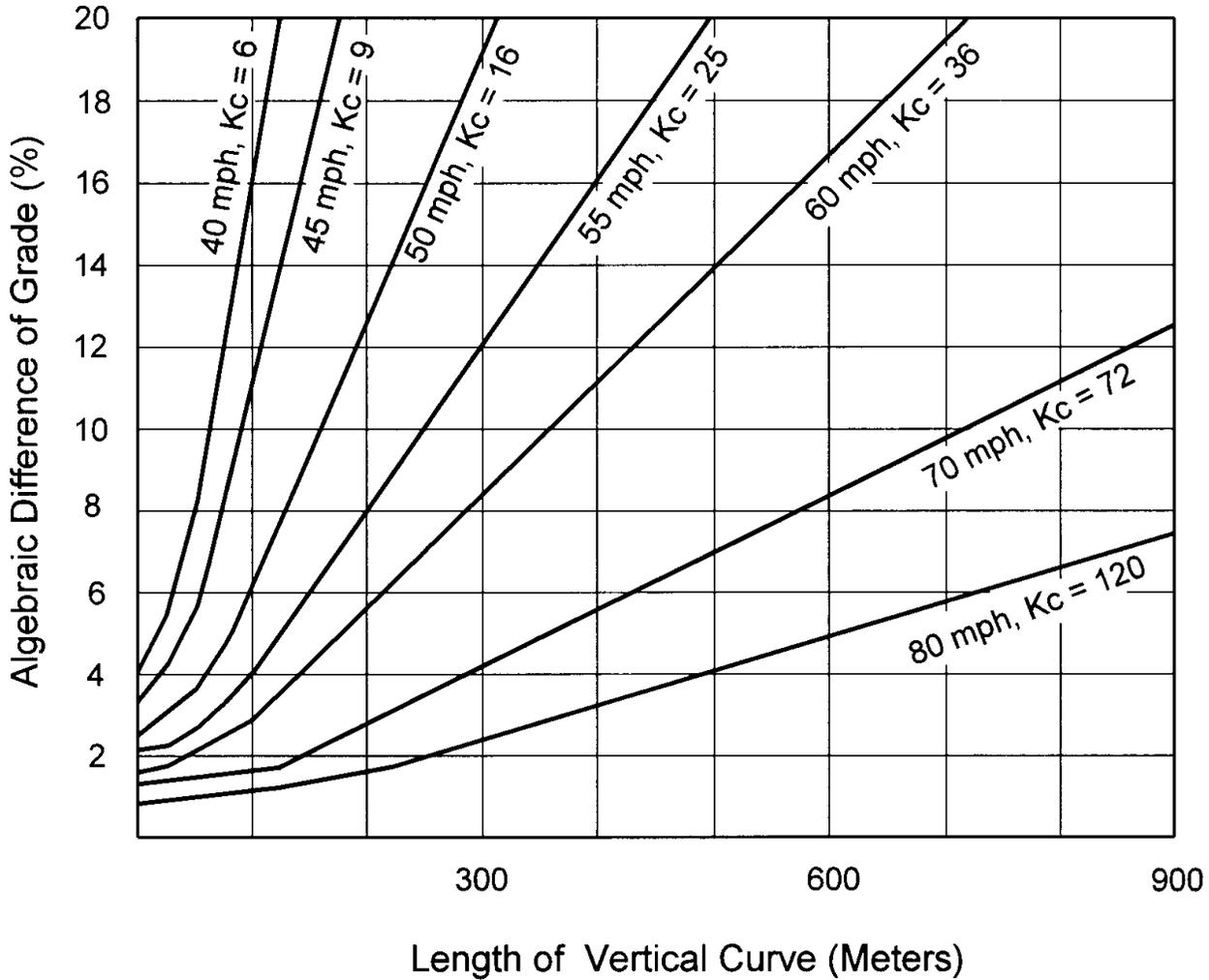
When the intersection of the algebraic difference of grade with the length of vertical curve is above the selected design speed line, corrective action must be considered.
