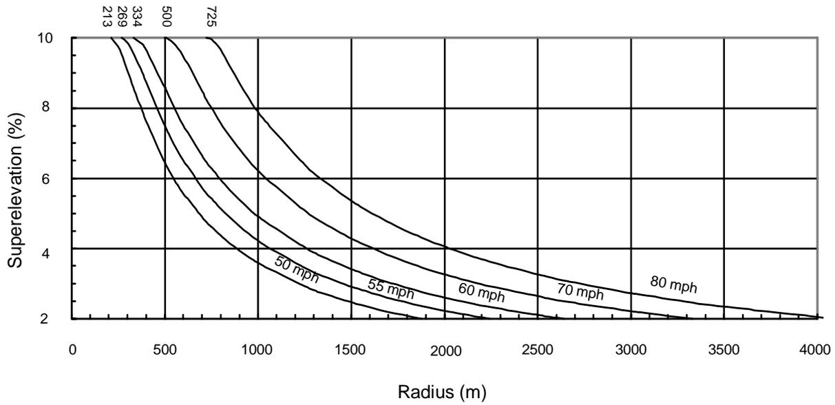
**Superelevation Rates (10% max)**
