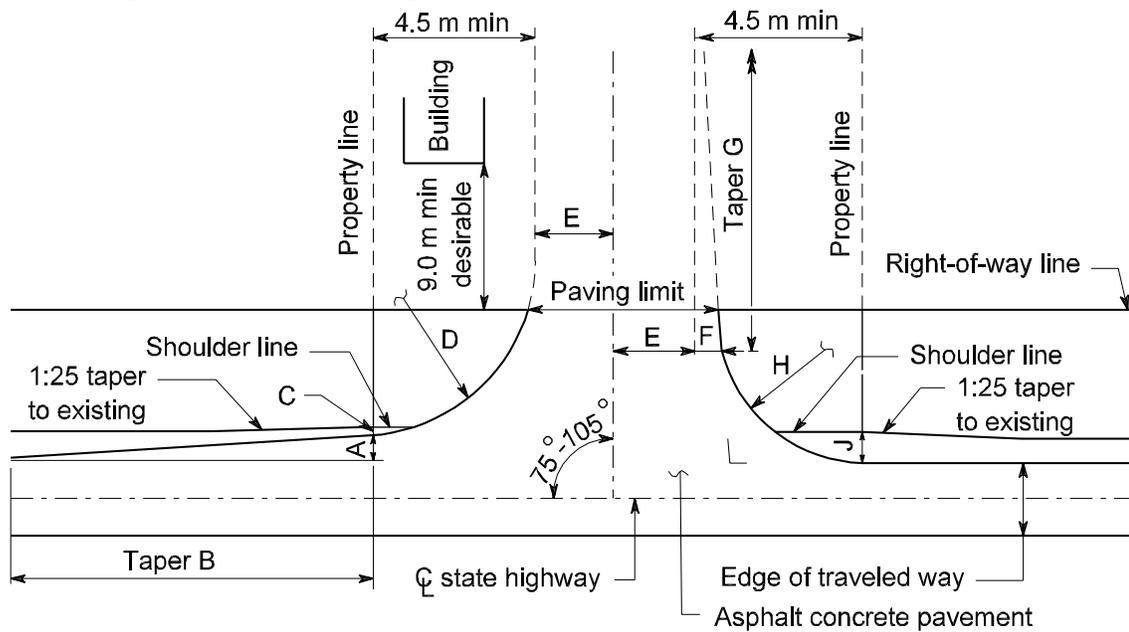
Note: Vertical curves between the shoulder slope and the approach grade not to exceed a 85 mm hump or a 50 mm depression in a 3.0 m chord.
