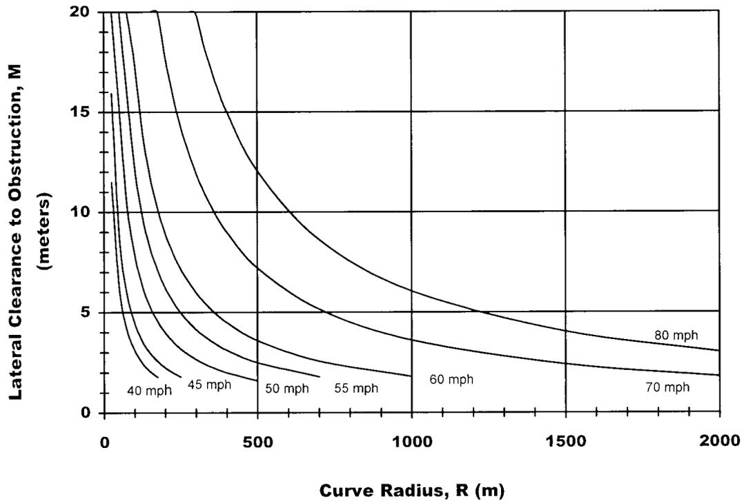
When the intersection of the lateral clearance (M) with the curve radius (R) falls below the curve for the selected design speed, corrective action must be considered.
