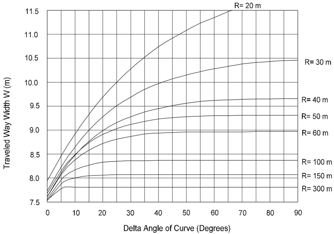
**Traveled Way Width for Two-Lane One-Way Turning Roadways**
