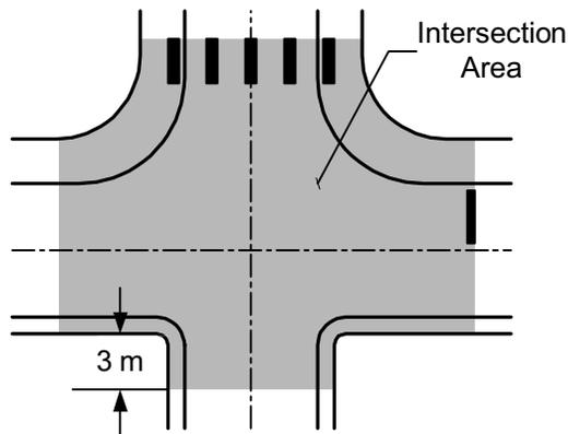
**intersection at grade** The general area where a state route or ramp terminal is met or crossed at a common grade or elevation by another state route, a county road, or a city street.
