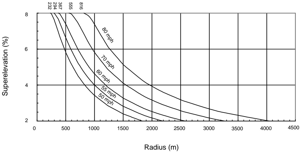
**Superelevation Rates (8% max)**
