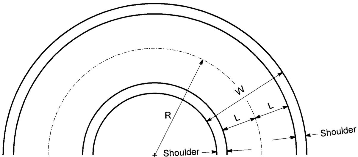
**Minimum Total Roadway Widths for Two-Lane Highway Curves
