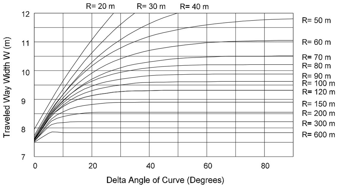
**Traveled Way Width for Two-Way Two-Lane Turning Roadways**
