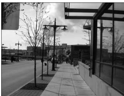
Sidewalk With Buffer Exhibit 1510-3
