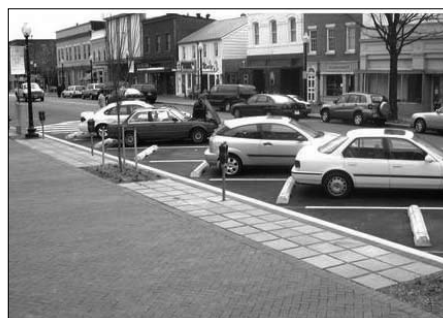
Sidewalk With Buffer Exhibit 1510-3
