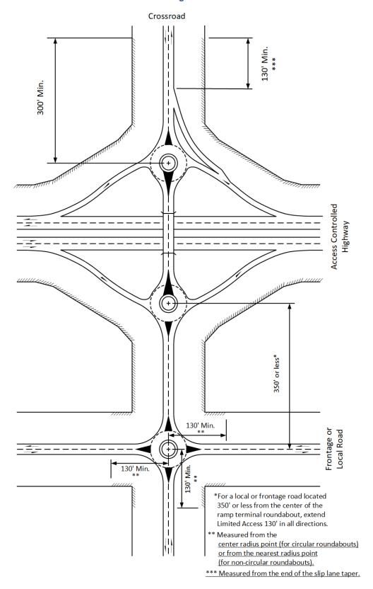
**Exhibit 530-4 Full Access Control Limits: Ramp Terminal with Transition Taper**
