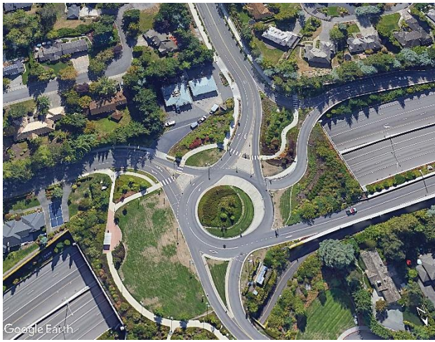
Five-leg roundabout with commercial property access driveways split between two approaches – 84 th Ave at SR520, Bellevue (Source: Google Earth)
