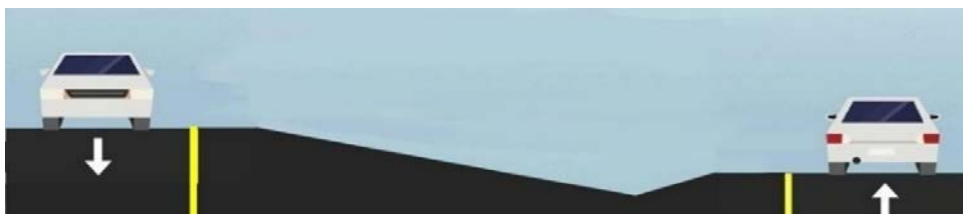
Exhibit 1232-3 Median Section without Median Barrier
