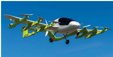
Advancements in drone technology lead to new transportation applications like this Kitty Hawk Cora eVTOL urban air mobility autonomous air taxi.
