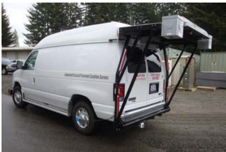
WSDOT's pavement monitoring van.
