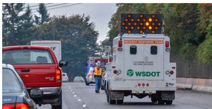
A WSDOT Incident Response unit uses its arrow board at an incident scene, alerting drivers of the need to merge. This technique protects emergency responders and drivers as well as helps manage traffic flow.
