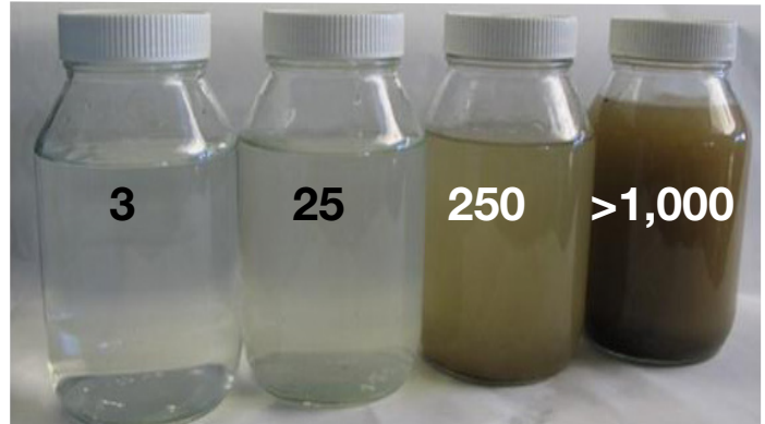
Water samples depicting Nephelometric Turbidity Unit levels. These are the units used to measure turbidity.
