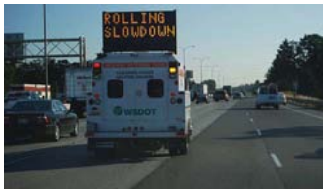
Some Incident Response vehicles are equipped with variable message signs (VMS) that can inform motorists of incidents ahead.
