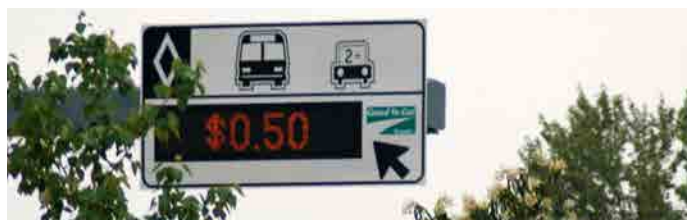
Toll rate displayed on overhead signs alert drivers to the current cost of using the SR 167 HOT lanes as a solo driver. High occupancy vehicles can always use the lanes for free.
