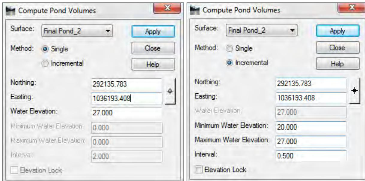
This tool generates volumes via two methods: (1) Single, and (2) Incremental. The **Single** method returns a single volume quantity up to a user defined elevation. The **Incremental** method computes volumes at different elevation increments.
