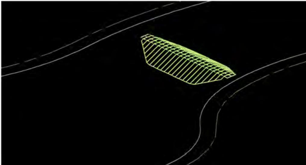
An access road to the first cell is a required design element and the process steps are similar to the cross berm design: create geometry, template, and model the Merge Pond, Berm, and Access Road surfaces to produce the final DTM.
