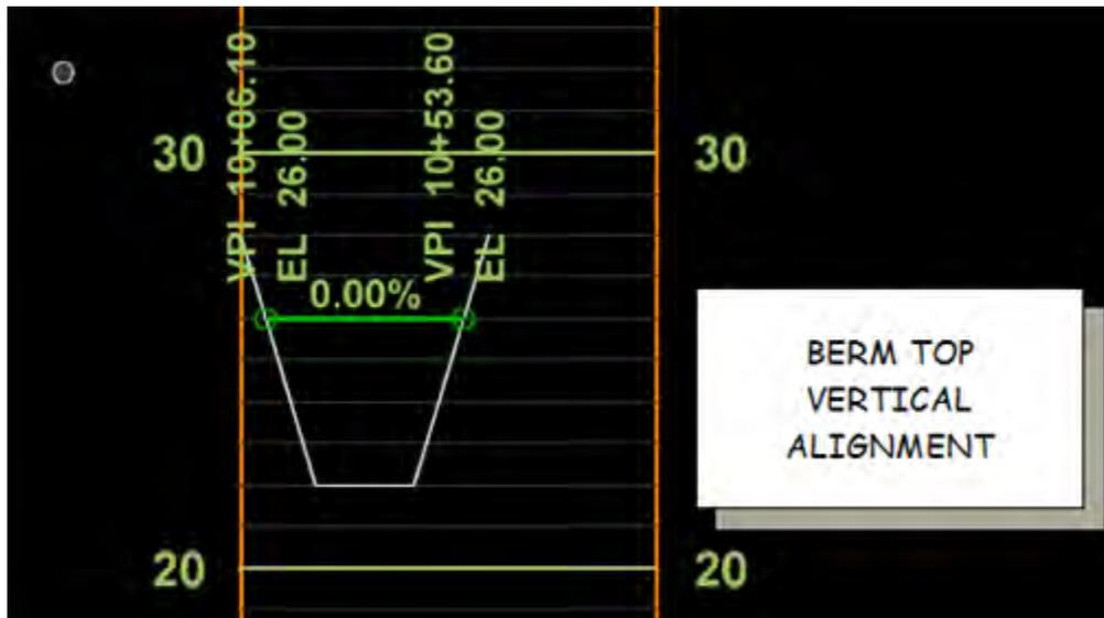
Create a template defining the berm top and end conditions targeting the Pond surface. Then create a corridor definition and model.
