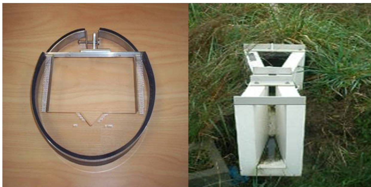
Figure 17 6-inch Thel-Mar-type v-notch weir (left) and 1-inch throated Parshall flume (right).
