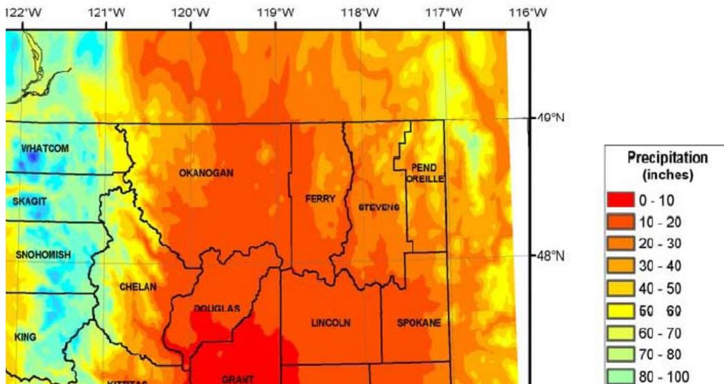
From the Isopluvial to Peak Intensity Factor chart in the FC.01 Natural Dispersion section of the HRM, we find the PIF for Spokane (climatic region 3) to be 2.03in/hr.
