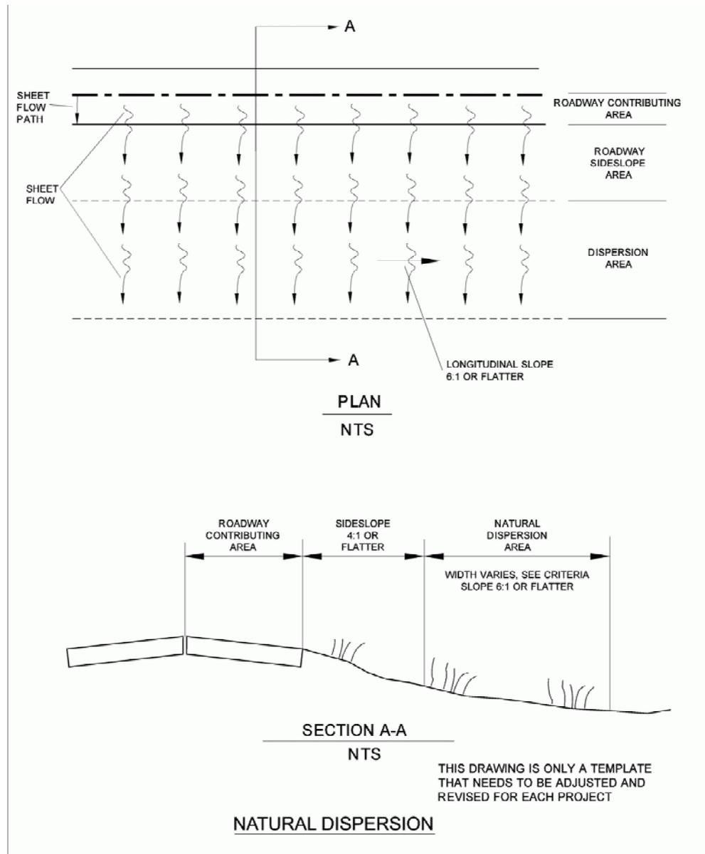
\*\*The dispersion area starts once the side slopes become 15% (6:1) or flatter. If the side slopes are already 6:1 or flatter, no buffer area is needed.
