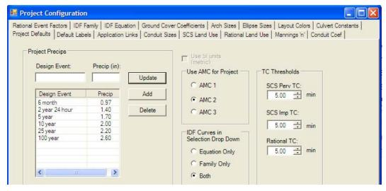
Of the tabs in the <u>Project Configuration</u> dialog box, the *Project Defaults* tab will likely be used the most by designers. This is where the precipitation values are set for each project location.
