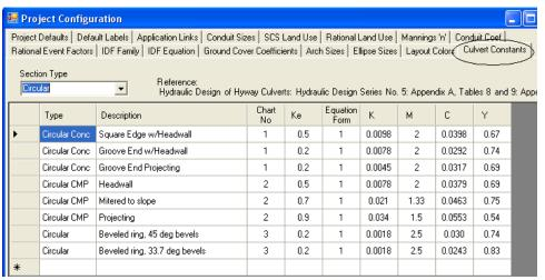
The *Culver Constants*<sup>1</sup> tab contains the Coefficient information used in the <u>Reach</u> Dialog Box pulldown menus for entrance losses. These values are based on the FHWA guidelines and can not be modified although new values can be added.
