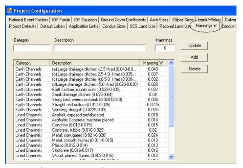
The *Mannings 'n'* and *Conduit Coef* tabs contains Manning's values directly from Appendix 4 of the Hydraulics Manual. These values can be selected from the pull down menu in the <u>Reach</u> Dialog Box. Use this tab to modify or add values that will more accurately reflect a project site.
