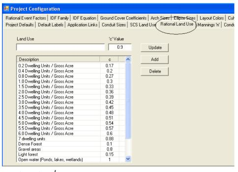
The *Rational Land Use<sup>1</sup>* tab, contains the coefficients for ground cover that are applied when calculating the Time of Concentration using the Rational Method. These values match the values found in section 2-5 of the Hydraulics Manual 2-5. This tab can be used to modify or add values that will better represent a project location.
