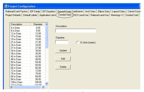
The *Conduit Sizes*<sup>1</sup>, *Arch Sizes*<sup>1</sup>, and *Elipse Sizes*<sup>1</sup> tabs are used to modify or add the default pipe sizes (the *Conduit Sizes* tab is shown above). These sizes and dimensions can be found in the Reach Dialog box pull-down menus to set pipe sizes. *Note the SI Units tab is only there to modify a design that is already been created in US units and then change to SI and the report will be printed in metric.*
