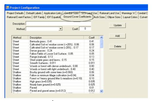
The *Ground Cover Coefficients*<sup>1</sup> tab, contains the default values for the type of flow (sheet, shallow, concentrated, etc) found in the <u>Basin</u> Dialog Box pulldown TC menus. Unique values can be modified or added here.
